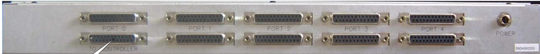
MX cable from one of the system controller MX bus connections. This cable overall length can not exceed 300'.
