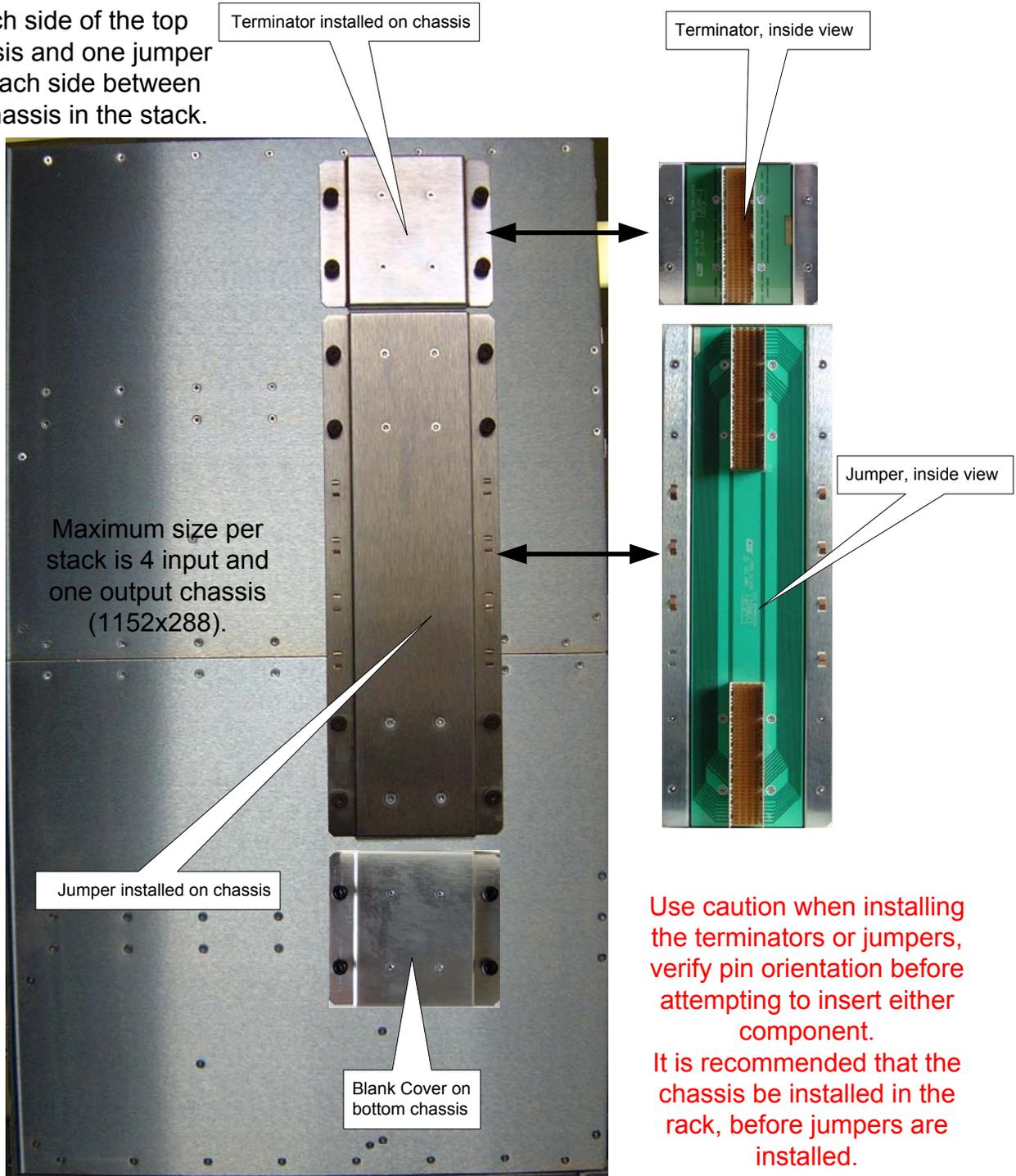
Use caution when installing the terminators or jumpers, verify pin orientation before attempting to insert either component. It is recommended that the chassis be installed in the rack, before jumpers are installed.
