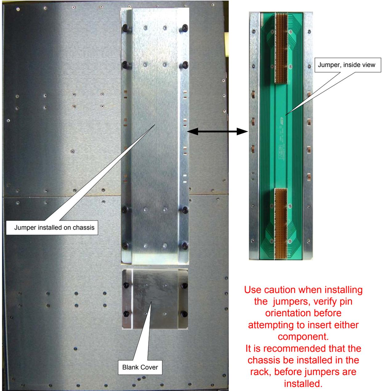
Use caution when installing the jumpers, verify pin orientation before attempting to insert either component. It is recommended that the chassis be installed in the rack, before jumpers are installed.
