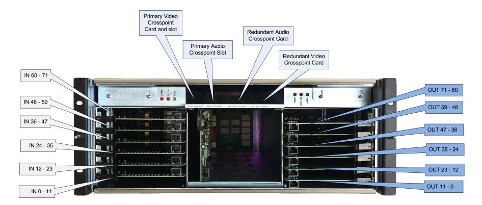
The above I/O layout contains Inputs 0-72 and is valid only when Crosspoint card (part #121337-2) is in use.
