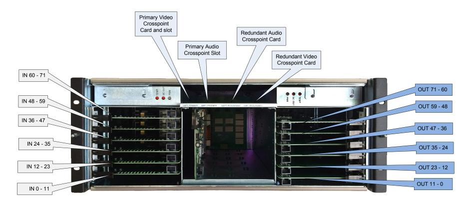
The above I/O layout contains Inputs 0-72 and is valid only when Crosspoint card (part #121337-2) is in use. (Outputs 0-131 are valid when Crosspoint card #121337-1 is in use.)
