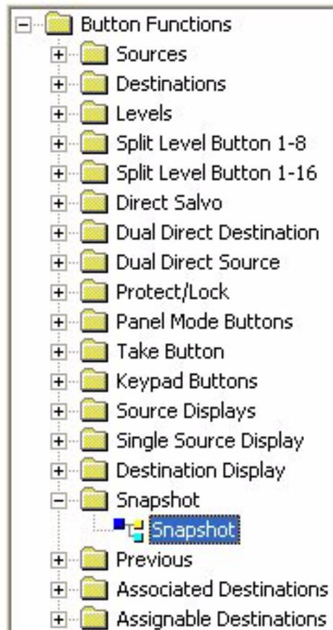
Snapshot buttons are used for defining a set of takes which can be triggered by pressing this button in the actual soft panel or retrieving a snapshot from the menu and taking it from there. These are only used with multiple destinations such as a monitor wall and are not to be confused with salvos. One or more of the outputs can be taken at the same time using a snapshot by retrieving the snapshot as a preset and then performing a take with the desired outputs by choice.
