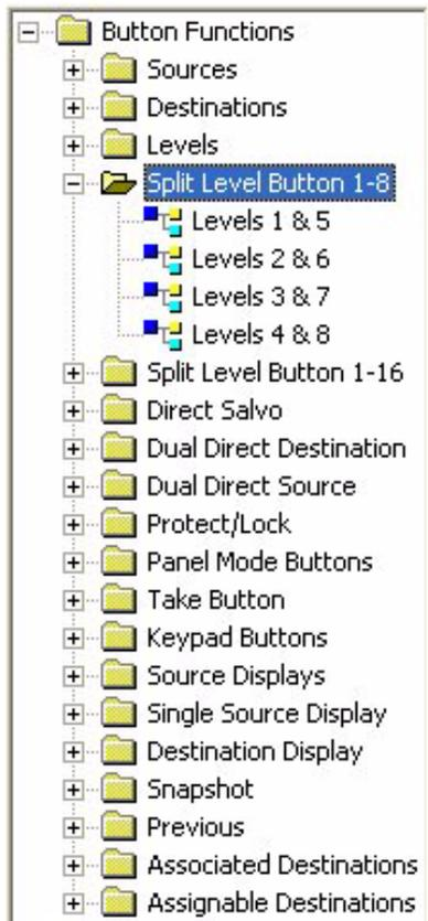
The split level buttons were designed to be used on the UCP-2, UCP-36, and UCP-72 panels. They give the user the ability to control 8 levels on 4 buttons. They should be used in conjunction with the “Panel Mode Buttons” and “Level Shift 1-4/5-8” button. This gives the user the ability to shift between levels 1-4 and 5-8.
