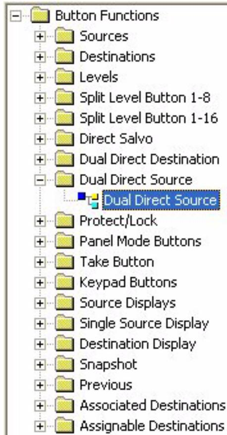
This allows the button to select between two different direct sources on one button. Use this button function in conjunction with the *Panel Mode Buttons/Source Shift* function. In conjunction with the 'Source Shift', the user can have two different sources on one button. This will double the number of direct sources this panel can control.
