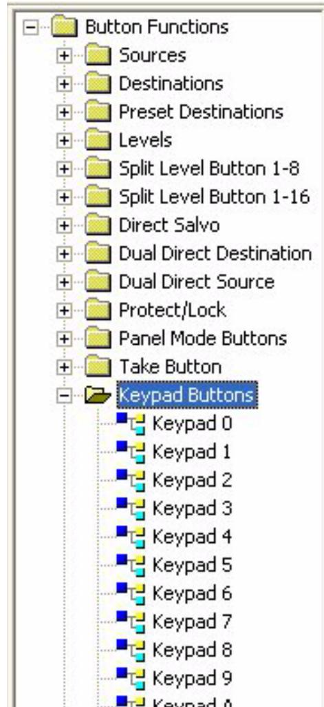
The Keypad layout buttons are mainly used on the UCP-2 panel. They define the keypad layout of 0 - 9, A - F, and 16 - 19.
