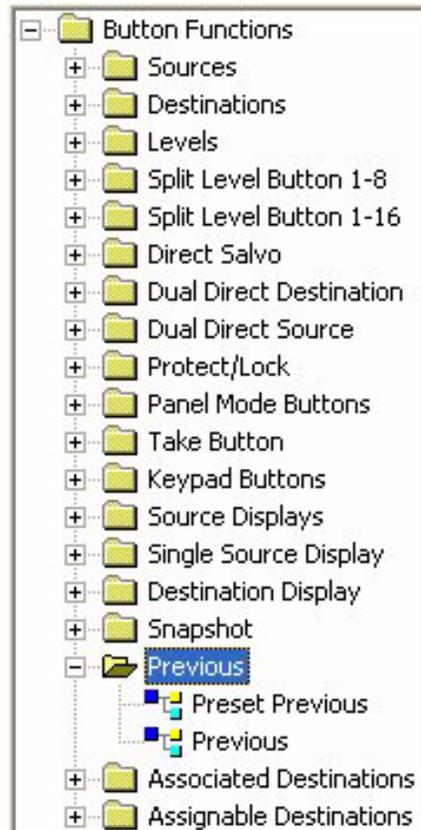
There are two options in the Previous folder. Both relate to reverting back to the previous switch after a take is made. This does not undo the current take but it literally goes back to the previous take made. The option called 'Preset Previous' shows the previous take in a blinking state before taking it, allowing the user the option to cancel or continue on with a Take. This mode also requires a Take button on the panel. The option called 'Previous' will perform the take without a prompt.
