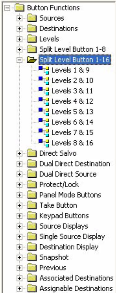
The split level buttons were designed to be used on the UCP-XY, UCP-SX, and the UCP-MX. They give the user the ability to control 16 levels on 8 buttons, and should be used in conjunction with the “Panel Mode Buttons” and “Level Shift 1-8/9-16” button. This gives the user the ability to shift between levels 1-8 and 9-16.
