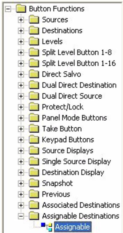
With this assigned as a destination button, the user can right click on the button in the panel to open the entire destination list of which they can select the desired destination.
