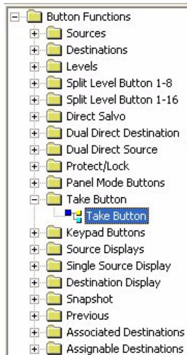
This will assign the take functionality to a button. After configuring a take, this button should be pressed to send the take to the controller.
