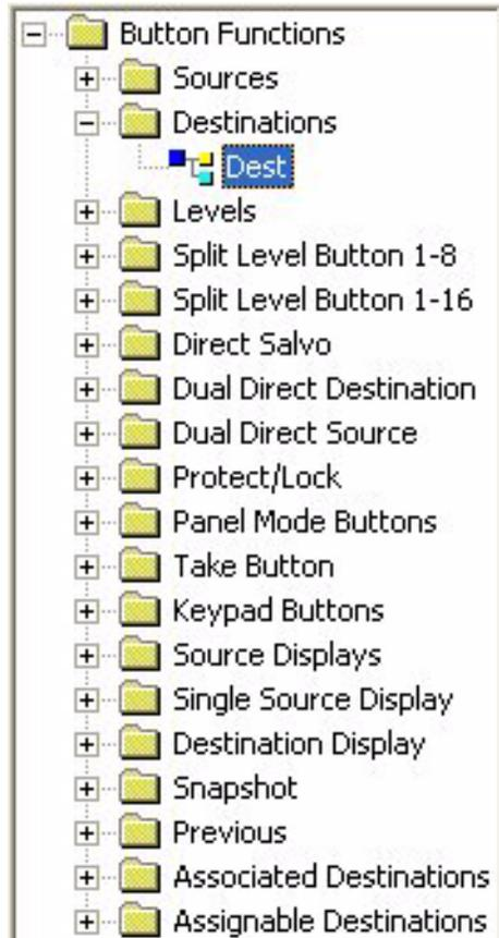
The Destination group will assign a button to control a given destination for this panel. The brightly lit destination is the current one that this panel will be switching to. If this panel does not contain any destination buttons, there should be a default destination assigned and labeled somewhere. In this way, the users can determine the appropriate output for this panel's control.
