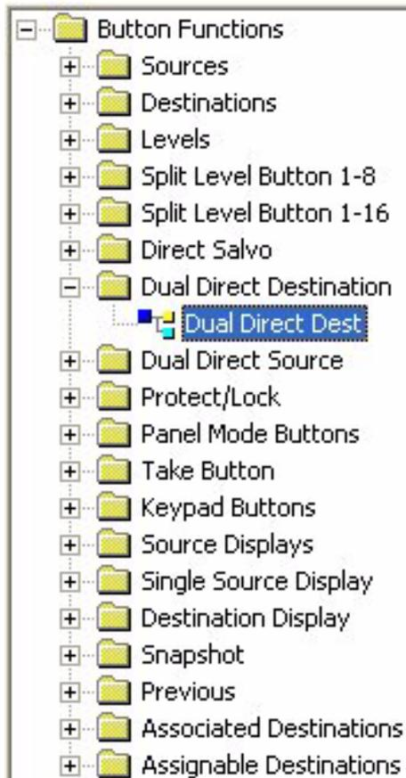
This allows a button to select the actual destination the panel will control. Assign (2) destinations to the button *after* assigning this function to the button. Once that happens, this button can be used to select the destination this panel will control.
