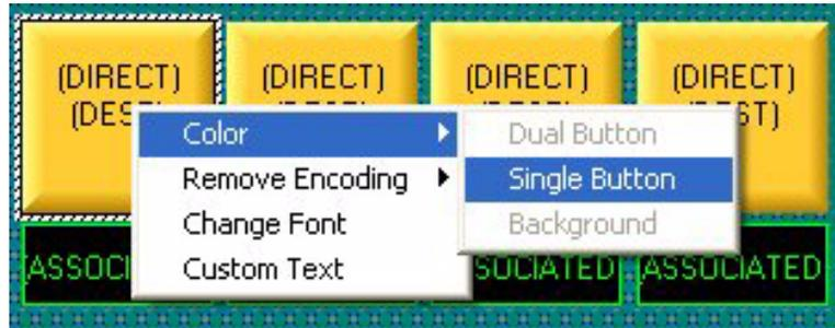
From that point forward, buttons are added to the display area by simply double-clicking the button type from the buttons folder. The buttons folder allows you to select and place content within the display area *only*.
