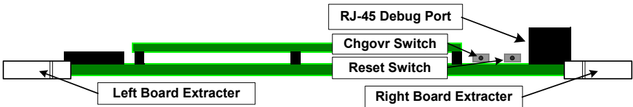
FIGURE 3-1. SC-4 Control Board Components – Front View
