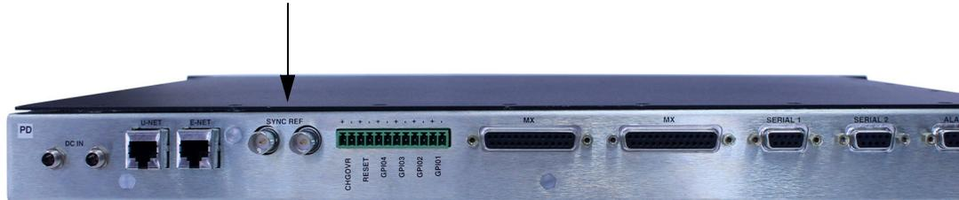
The sync ports should be fed with analog black burst signals, either NTSC, PAL, or Tri-Level. **Do not connect digital SDI or HD-SDI signals to these ports.**
