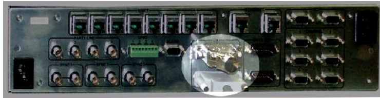
Figure 3-8. The MX-Bus Connectors (SC-4 rear)
