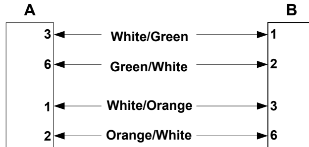
Figure 3-11. Pinouts for a Crossover Ethernet Cable
