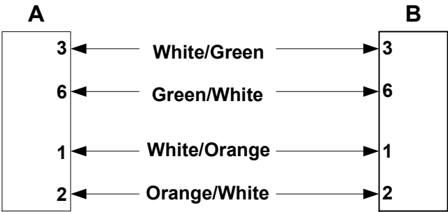
Figure 3-13. Pinouts for a straight-through Ethernet cable
