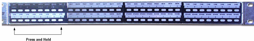
Figure 6-18. Button combo for dip switch setting
