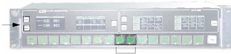
Figure 3-24. UCP-MMA Panel - Beep and Click volume adjustment
