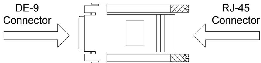
**FIGURE 2-13. D-subminiature to RJ-45 Adaptor**
