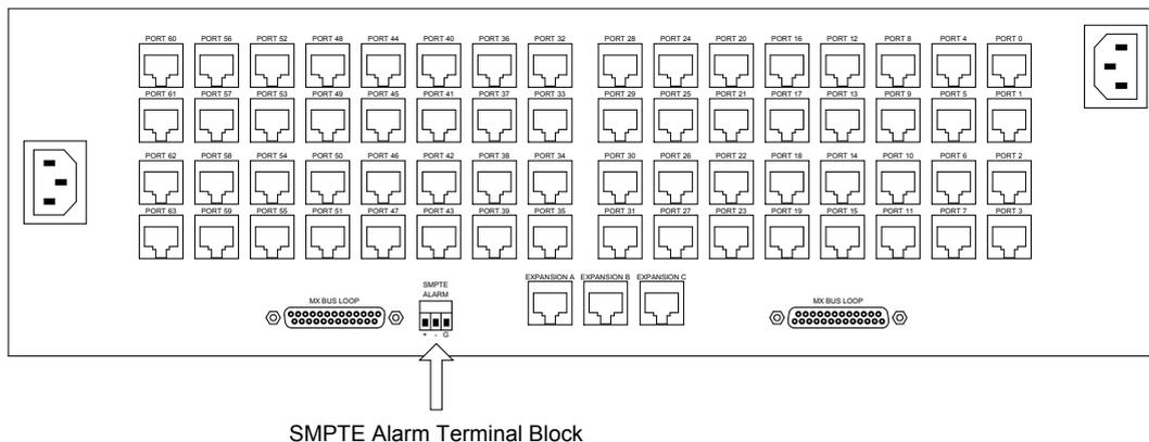
**FIGURE 2-21. Utah-400 Data Router – External Alarm Connection**
