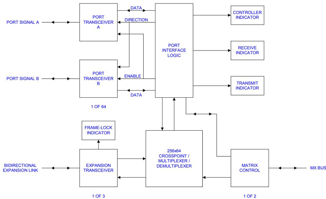
**FIGURE 1-1. The Utah-400 Data Matrix Block Diagram**
