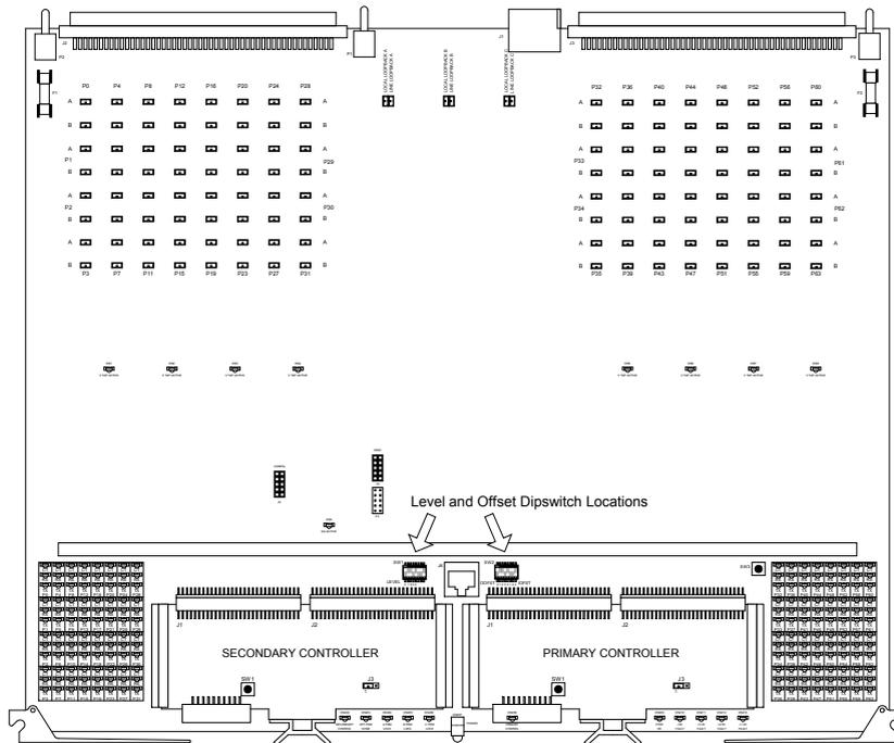
FIGURE 2-8. Main Board Assembly Dipswitch Locations
