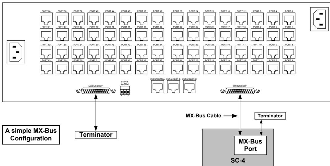
FIGURE 2-5. The MX-Bus Connection to an SC-4 Controller
