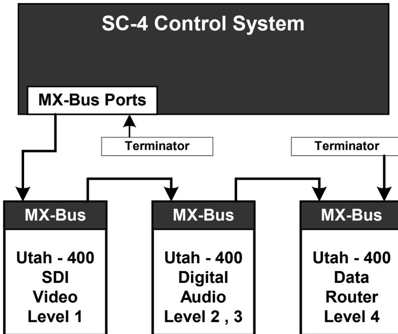
FIGURE 2-6. Block Diagram of an MX-Bus Daisy Chain
