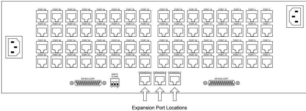
FIGURE 2-17. Utah-400 Data Router Rear Panel Expansion Ports
