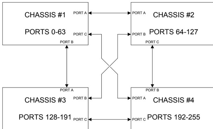
**FIGURE 2-20. Utah-400 Data Router – 4-Chassis System**
