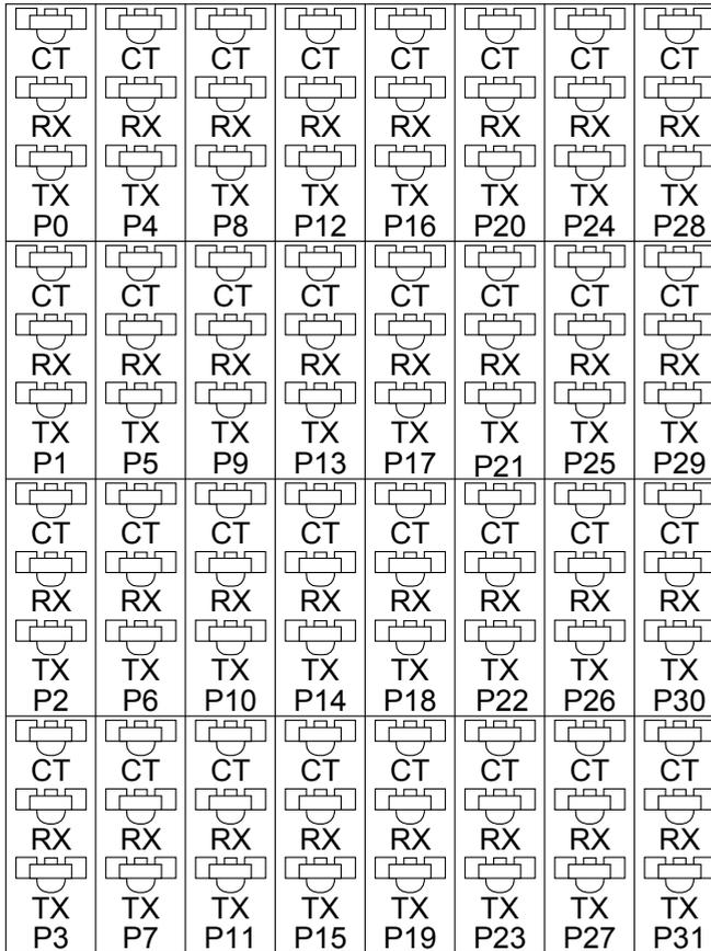
FIGURE 3-2. Port Status Indicator Array – Ports 0-31
