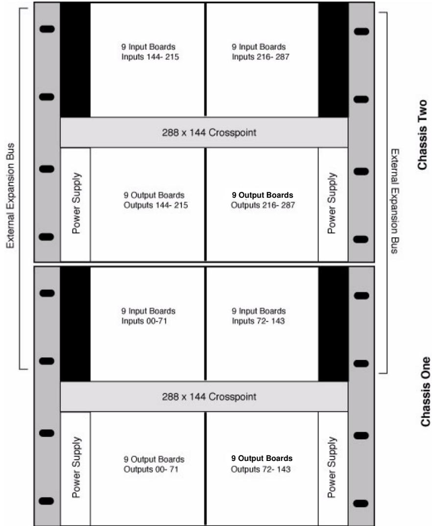
FIGURE 1-5. 288x288 SD/HD Chassis (non-expandable)
