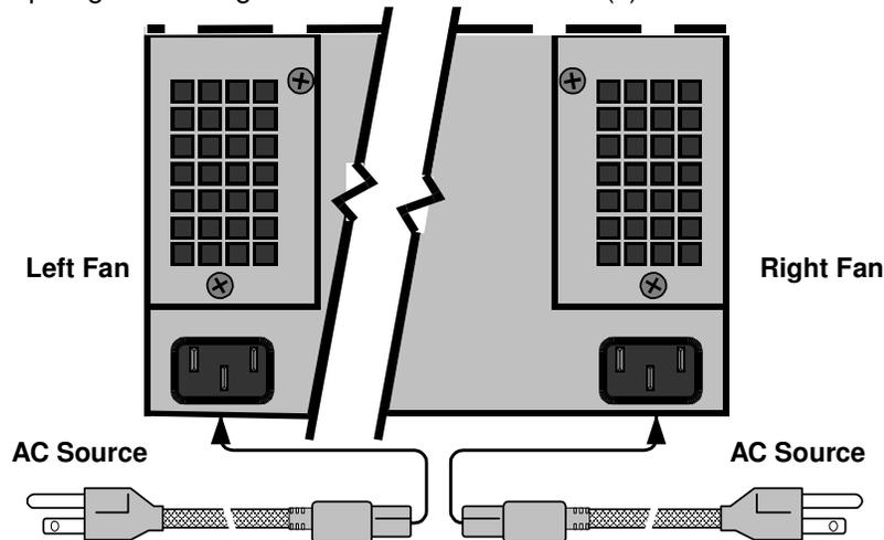
FIGURE 2-17. Utah-400 Power Connections
