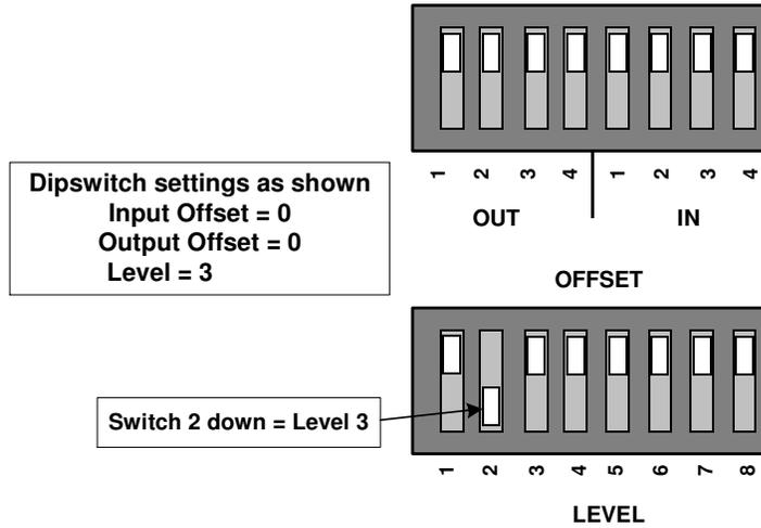
FIGURE 2-10. Utah-400 Configuration Dipswitches as they appear on the Crosspoint Carrier Board
