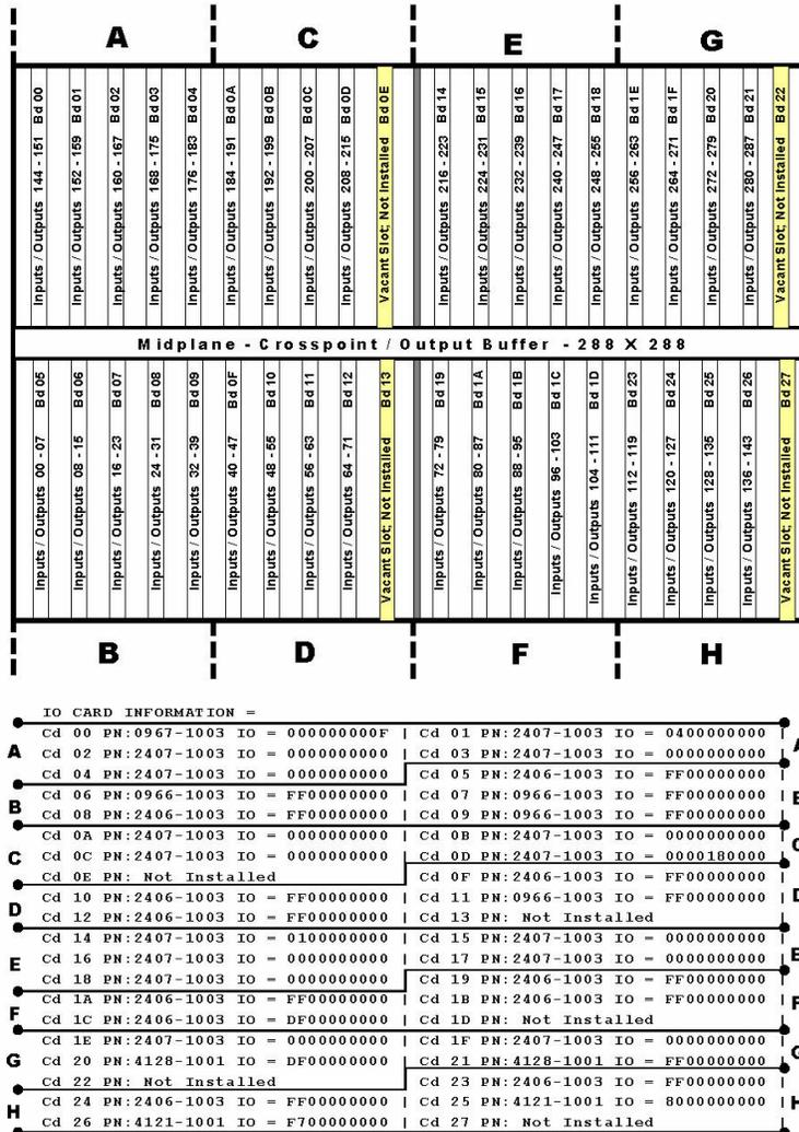
FIGURE B-8. I/O card information - locator diagram
