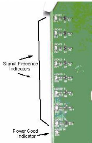
**FIGURE 4-12. Digital Video to Analog LED Indicators**
