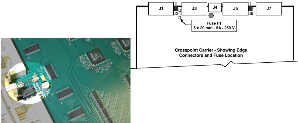
**FIGURE 4-35. Crosspoint board fuse assembly**
