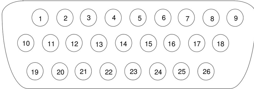
**FIGURE 2-15. DB-26 High-Density Male Connector**
