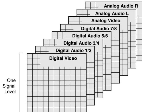
Signal routers are typically much larger than a 10 X 10 matrix, depending on user needs. Each signal level may also have different sizes of matrices and do not all need to be the same size.
