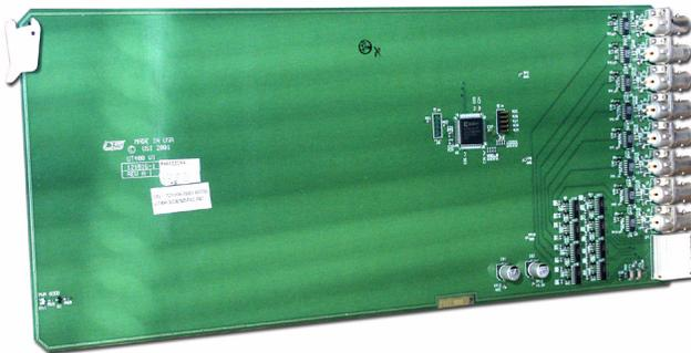
**FIGURE 4-1. SD Video Input Board**
