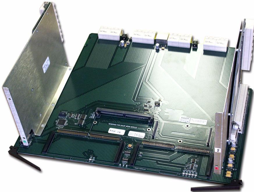
**FIGURE 4-22. Output Buffer card**
