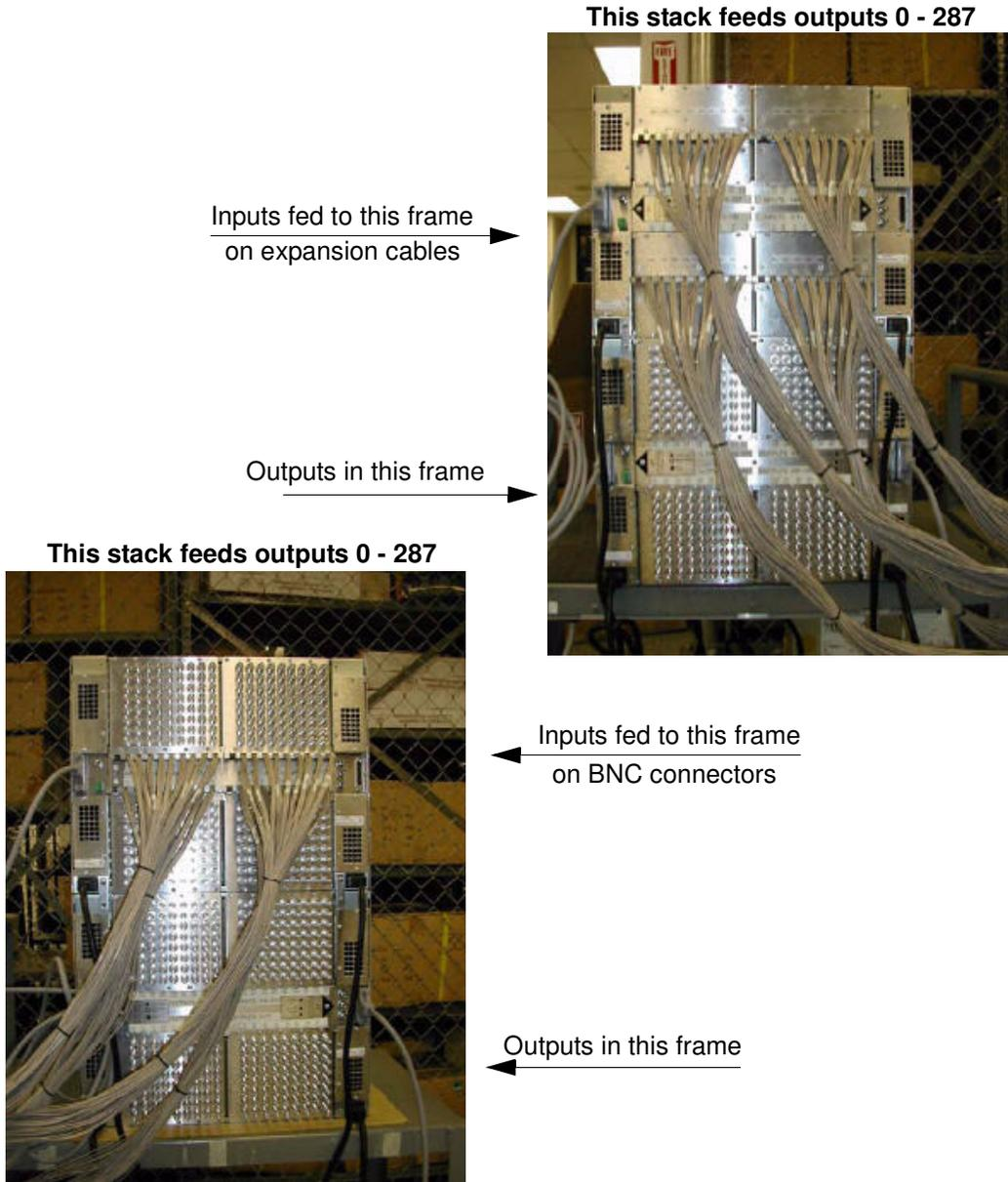
FIGURE D-8. Stack to Stack Expansion Views
