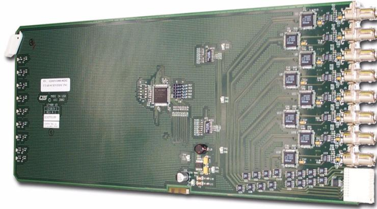
FIGURE 4-9. SD (Multi-Rate)Output Board
