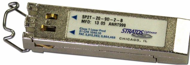
**FIGURE 4-16. SP2T - Transmitter module**
