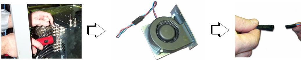
**FIGURE 3-4. Fan alarm, and device location**
