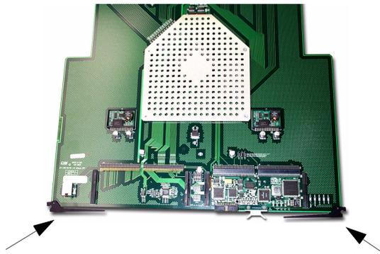
**FIGURE 3-3. Crosspoint Board Replacement and Removal**
