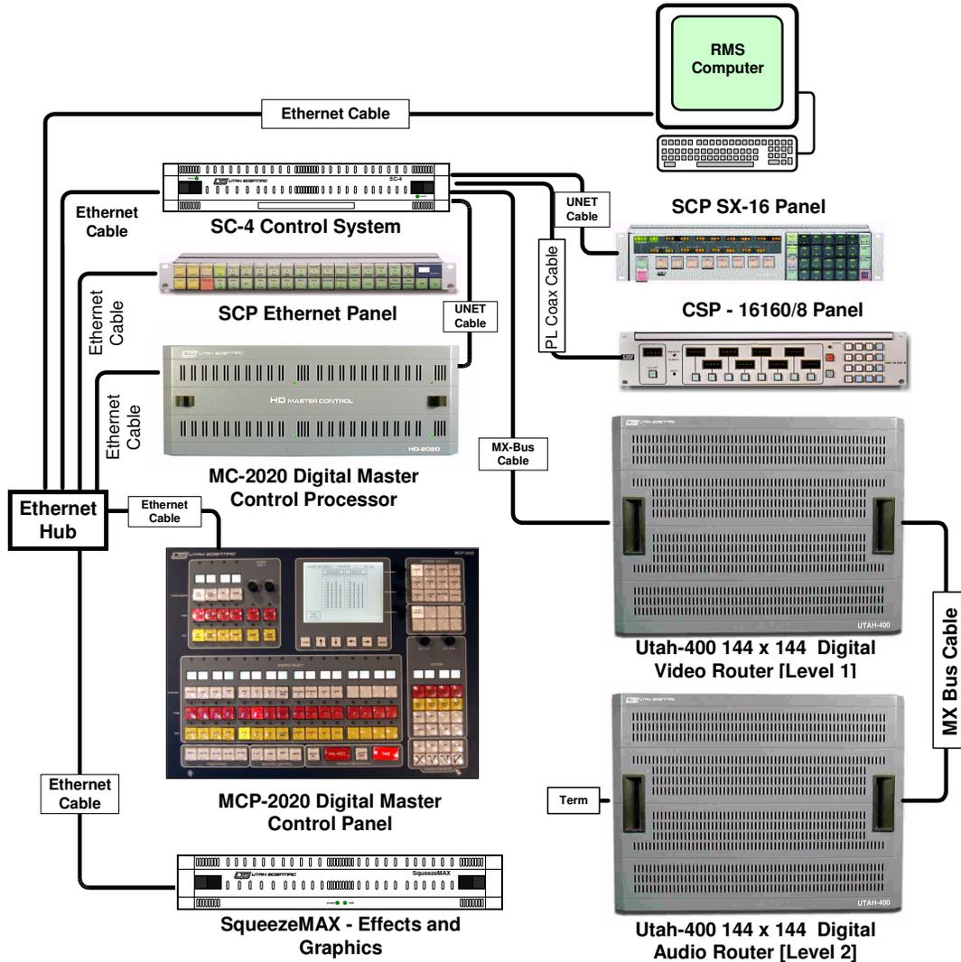
FIGURE 3-1. Utah 400 SC-4 for Utah-400 and MC/MCP-200
