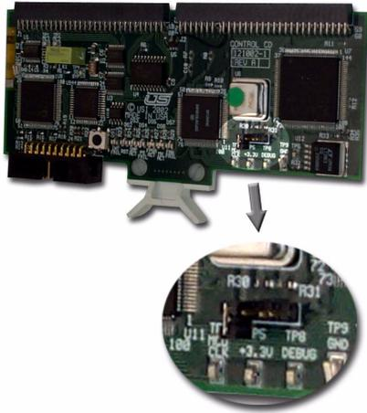
**FIGURE 4-21. Video crosspoint module jumper location**
