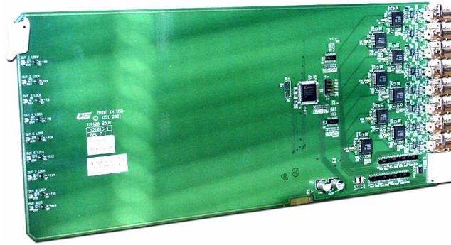
**FIGURE 4-8. SD Output Board**
