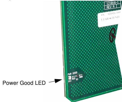
**FIGURE 4-11. SD and HD Output Power Good LED**
