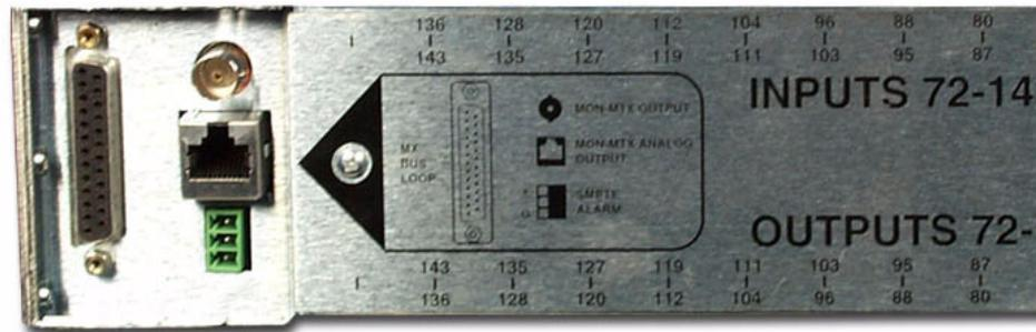
**FIGURE 4-25. Audio Midplane's RJ-45 connection**
