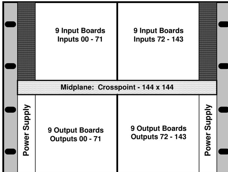
FIGURE 1-2. The Utah-400 144 x 144 Configuration
