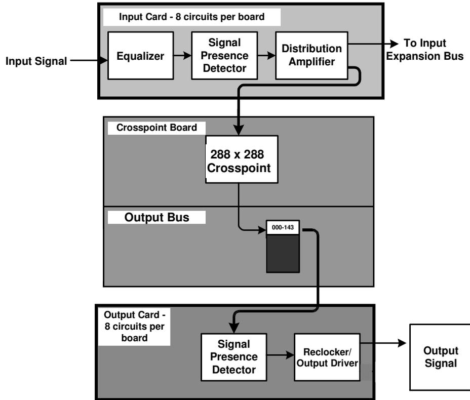
FIGURE 1-1. The Utah-400 Matrix Block Diagram
