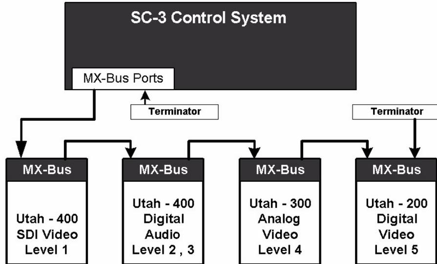
FIGURE 2-7. Block Diagram of the MX-Bus Daisy Chain.
