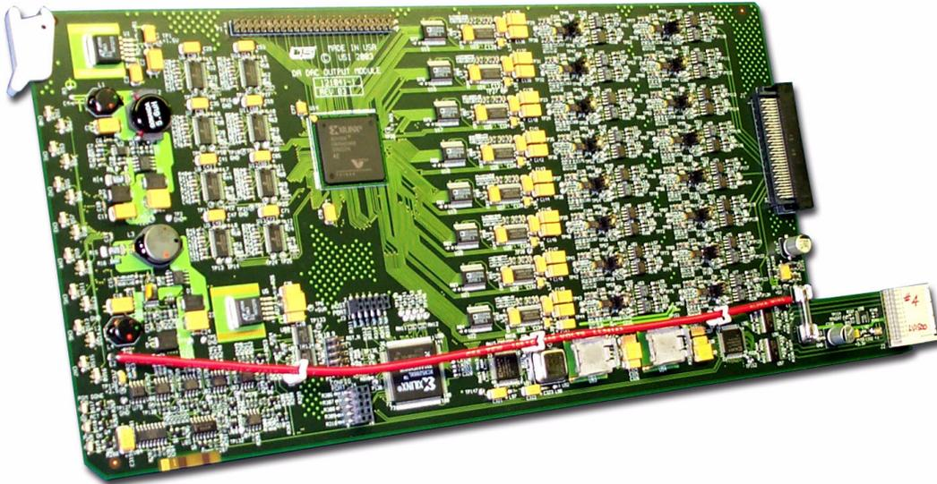
**FIGURE 4-32. DAC Output Module**
