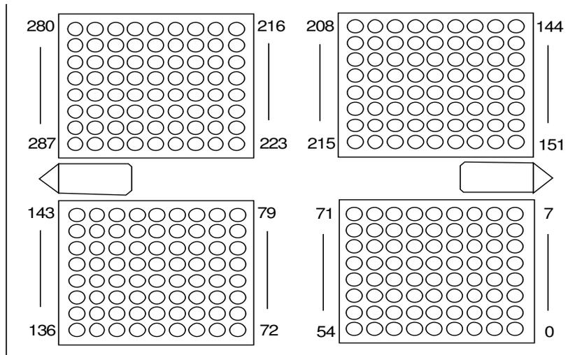
FIGURE 2-13. Unbalanced Digital Audio/Digital Video Output Connector Matrix
