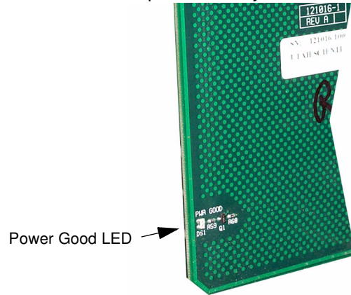
FIGURE 4-11. Video Output Power Good LED
