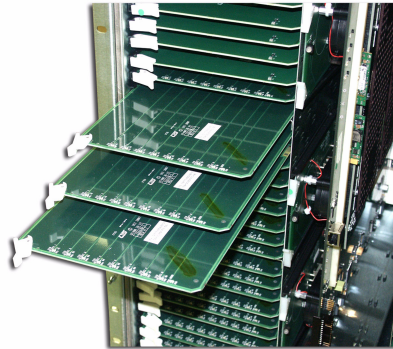
FIGURE 3-5. Input/Output Board Replacement and Removal
