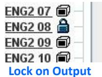
Clear will remove all protects and locks from that output. Double click on any output and it will change to the tabular status window and show all the levels and sources that are switched to that output as well as any locks or protects.
