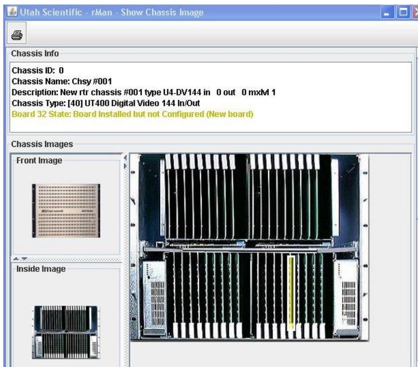
'Board' – these are position numbers of each I/O card when viewing the chassis. The numbers go top to bottom and left to right beginning with 1. All items will be underlined which indicates that they can be viewed. If the card has any issues or is removed, it will status red. If the slot is empty from when the last SC4 update happened, it will status blue. If a card is added to an empty slot since the SC4 was last updated, it will status yellow.
