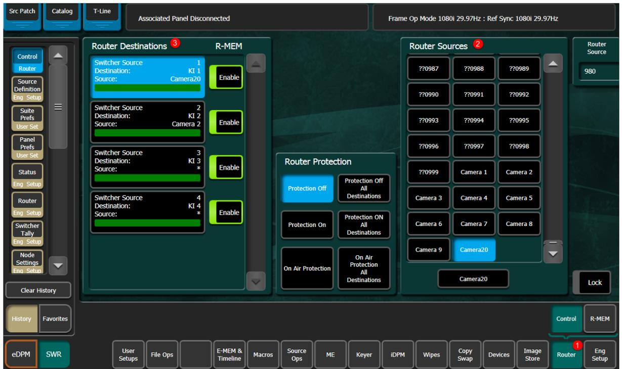
NOTE : All name changes require routing of the destination to change in vsmStudio. The connection will only be made from K-Frame to update names after the status of the routed crosspoint has been changed.
