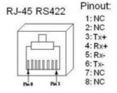
Connectors on rear side of UMD for serial data:
