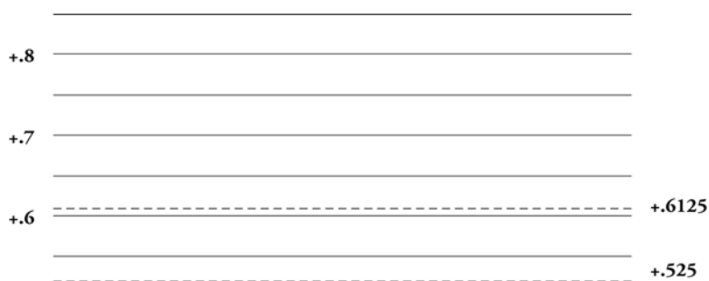
Figure 3-9. RGB and YCbCr Zoom 700 mV Graticule
