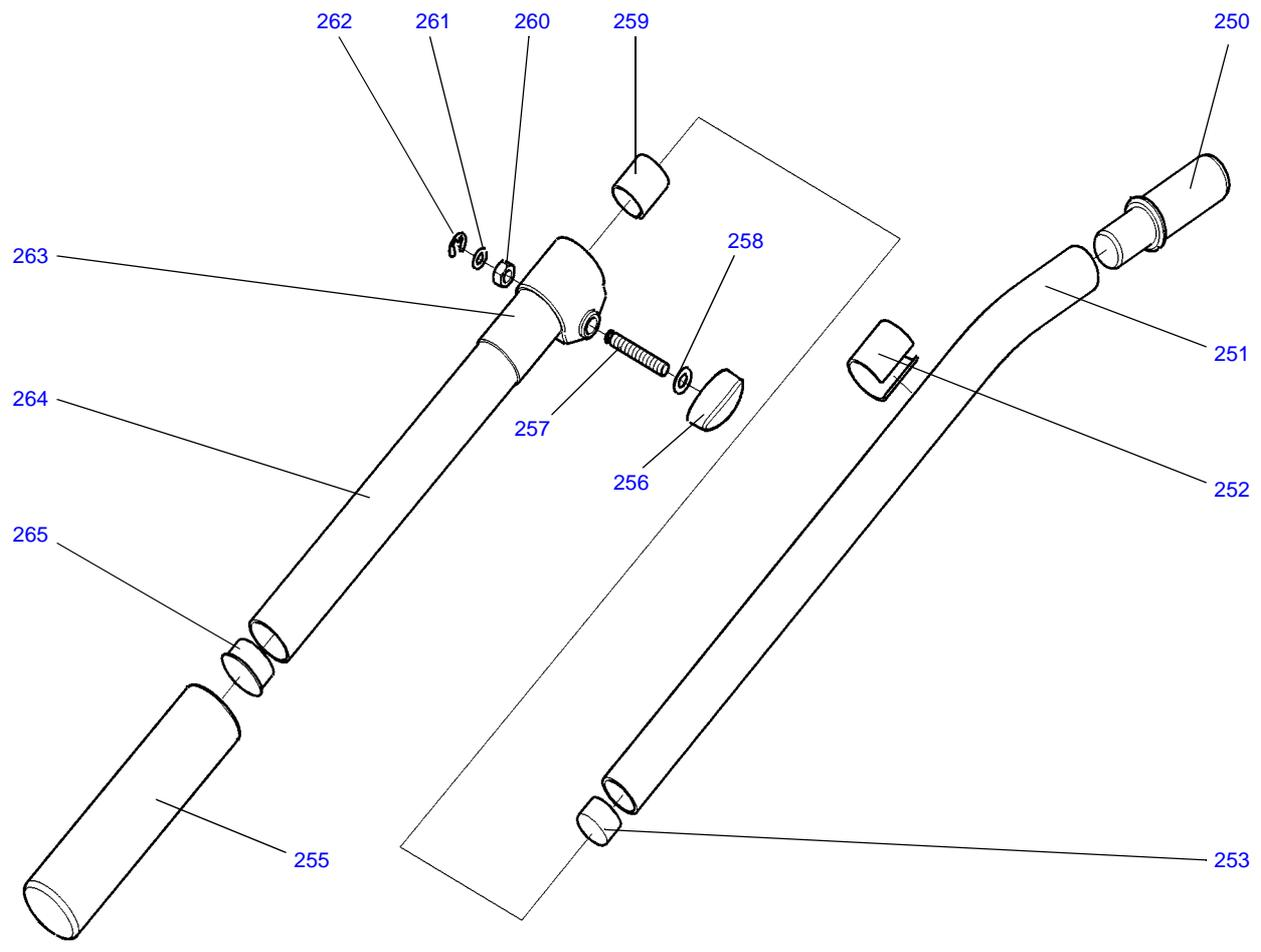
Fig 6.11 Pan Bar Assembly
