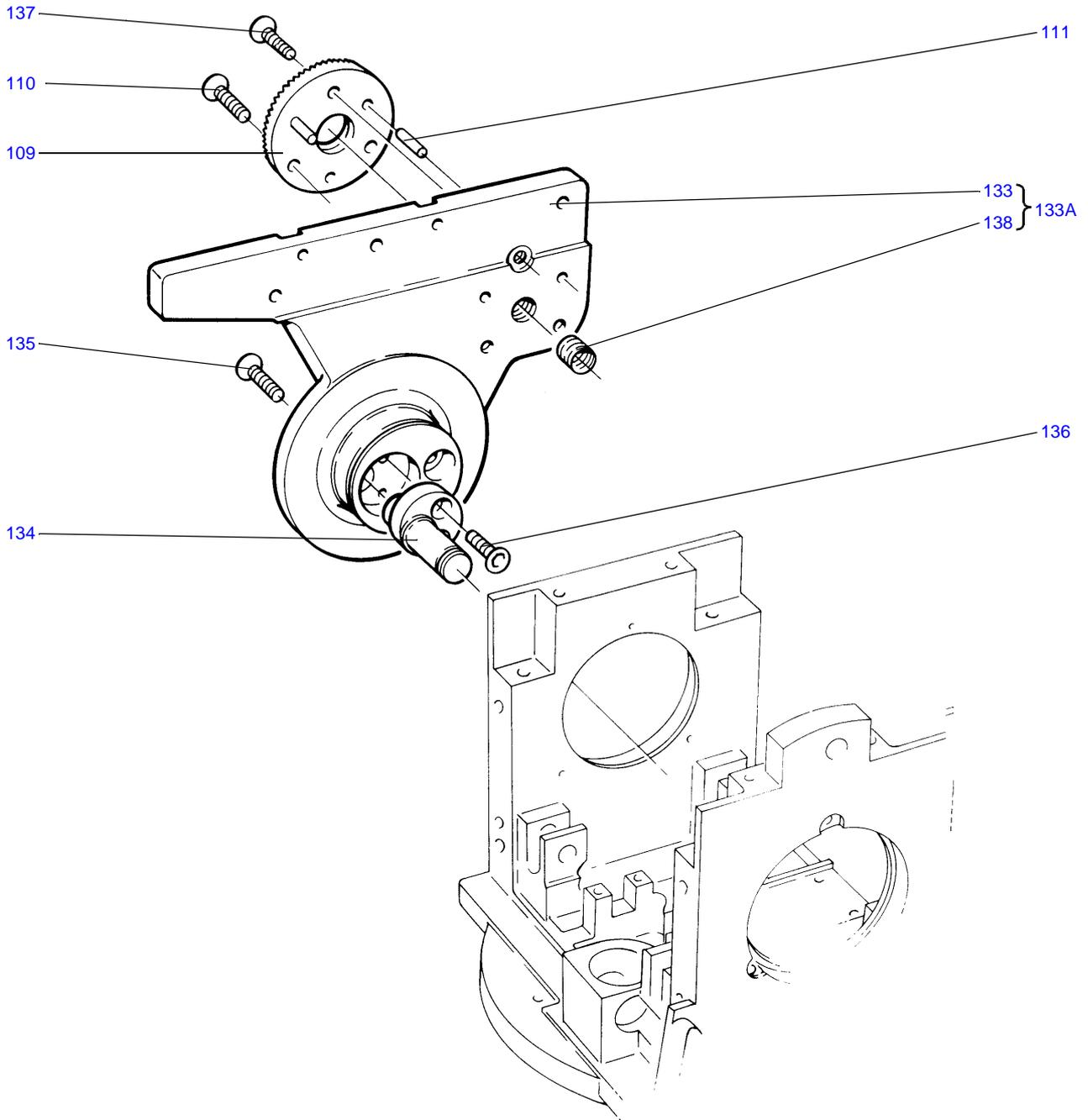
Fig 6.4 Side Plate Assembly
