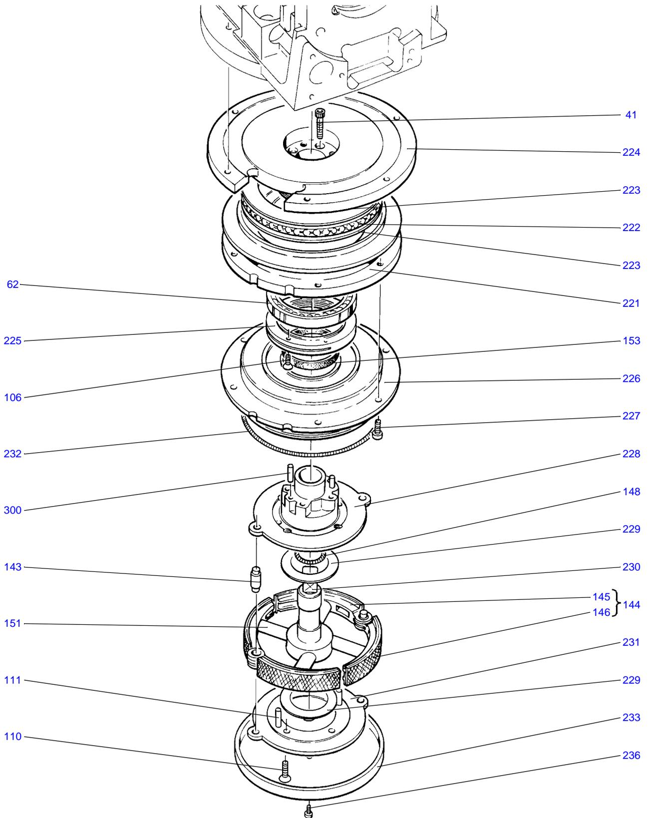
**Fig 6.9 Pan Drag Unit Assembly**
