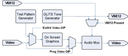
Figure 16 V6811 Block Diagram
