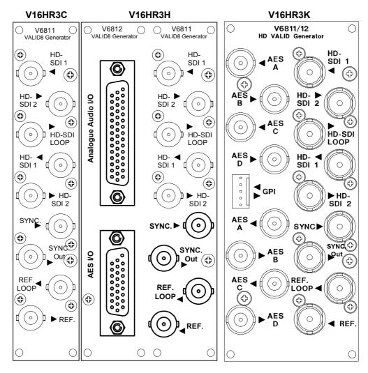
Figure 1 VALID Rears (V16HR3C & V16HR3H & V16HR3K)
