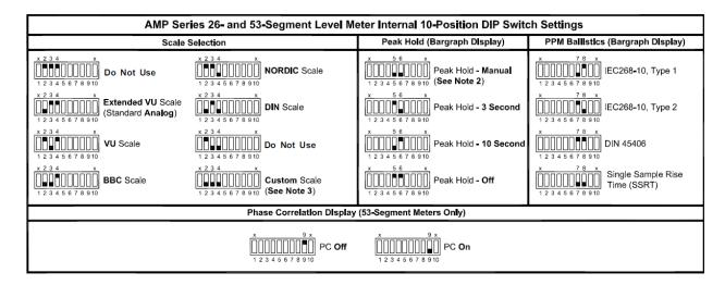
Switch positions 1 and 10 are not used and should be left at the factory set position.
