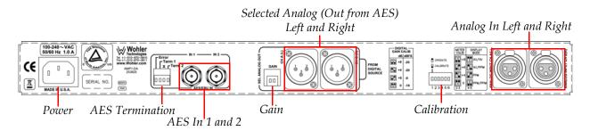
• **Power**: Attach a standard IEC-320 power cord between this connector and mains power (100 - 250VAC, 50/60 Hz). The front panel Power LED will glow green to indicate operating voltages are present.
