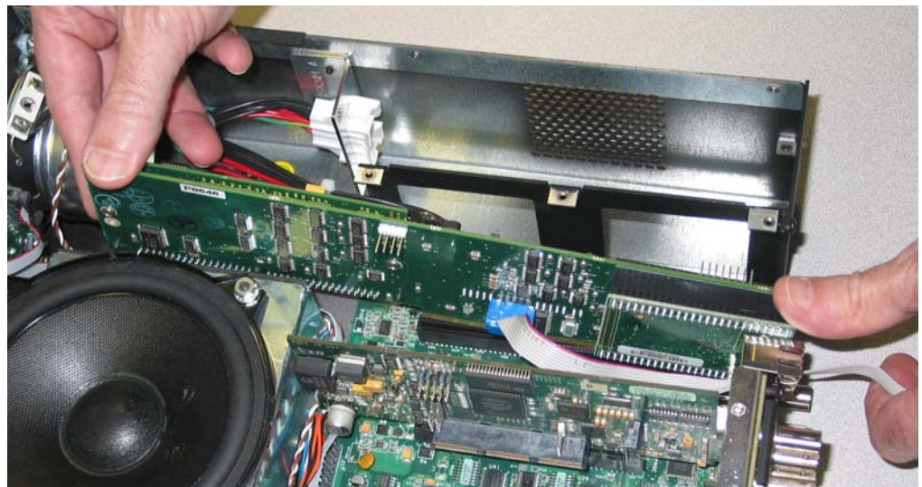
Figure 3–18 Re-Seat System Control Board
