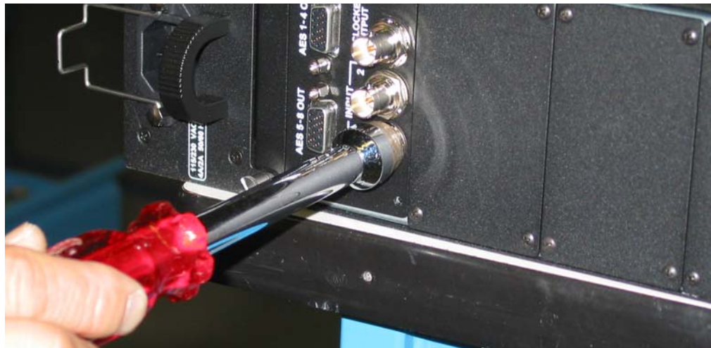
Figure 3–25 Tightening the BNC Nuts
