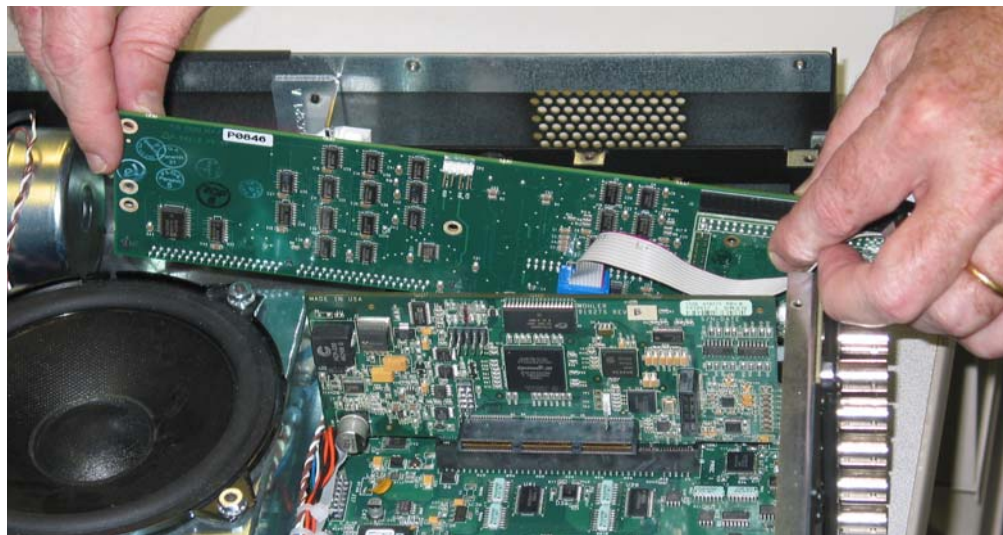
Figure 3–11 Remove System Control Board
