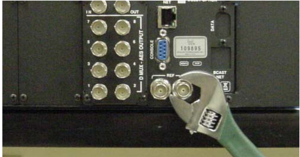
Figure 3–9 Remove Nuts and Washers
