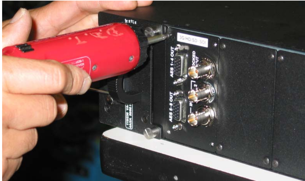
Figure 3–24 Tightening the Rear Panel Screws
