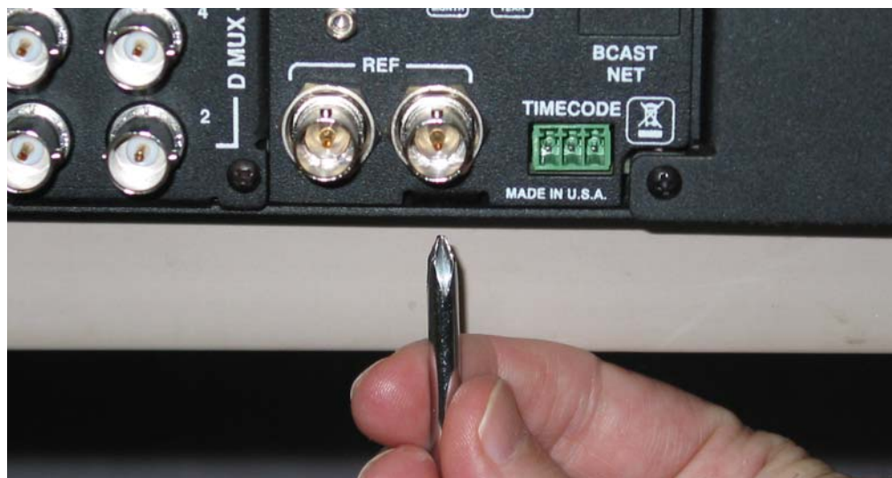
Figure 3–8 Remove Bottom Screw
