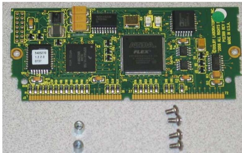
7. Remove the new Dolby D/E Card from its shipping container being careful to remain grounded. [Figure 8–11](#) above illustrates the card and the two standoffs (left) and the four screws (right).
