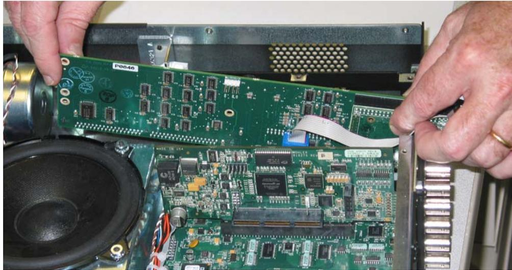
6. Gently tilt the system board out of its slot and remove it from the monitor as shown in [Figure 8–10](#) above.
