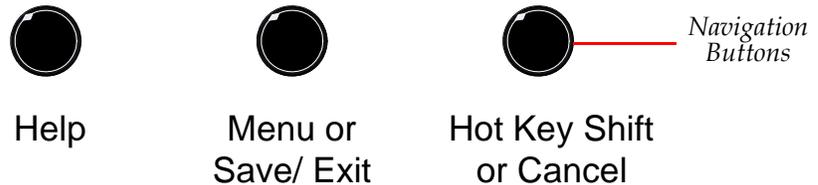
The functions of the navigation buttons can change depending upon the menu that is currently displayed. While the left button always generates context-sensitive **Help**, the function of the center and right buttons will vary. Usually the function of the center button is **Save/ Exit**; the function of the right button is usually **Cancel**.
