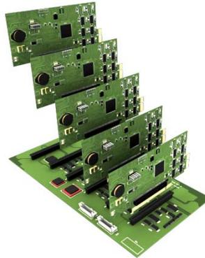
Note that you can add any of the I/O modules (listed in [Table 8–1](#)) or multiples of I/O modules, in any order.
