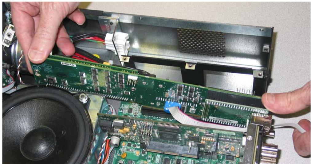
13. Firmly press the system control board back into its slot so that it is securely connected as shown in [Figure 8–17](#). Generally, this board does not snap in.
