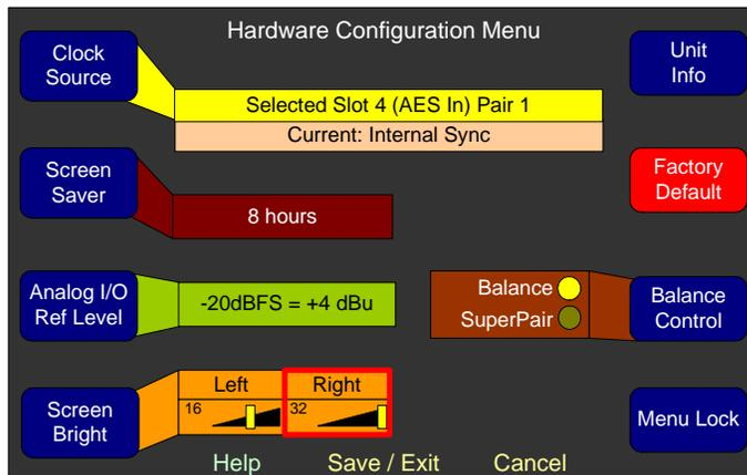
1. Turn the **Balance Control** knob to select **SuperPair** instead of **Balance**.
