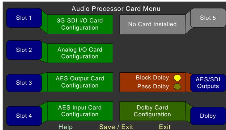
**Slots 1 through 5:** Each occupied slot displays the name of the card in that slot. Press the knob of the corresponding card to display the **Configuration Menu** for the card in that slot. If a slot is empty, the label will be gray and disabled, no card name will appear, and the knob will have no function. Rotating the knob does nothing; select the card by pressing the knob. Refer to the [AES/Analog Output Configuration Menus on page 91](#) for configuration option examples.
