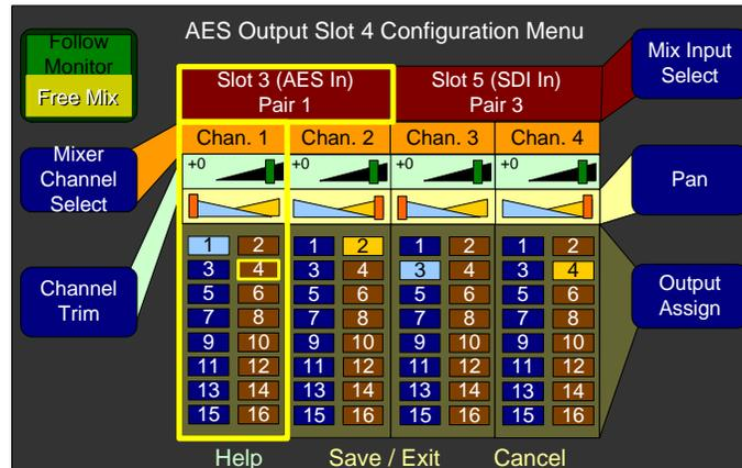
1. Press the **Follow Monitor / Free Mix** control to select **Free Mix**, as shown in [Figure 3-21](#) above.
