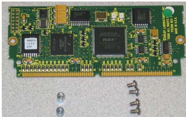
8. Remove the new Dolby D/E/DD+ Card from its shipping container being careful to remain grounded. [Figure 6-14](#) above illustrates the card and the two standoffs (left) and the four screws (right).
