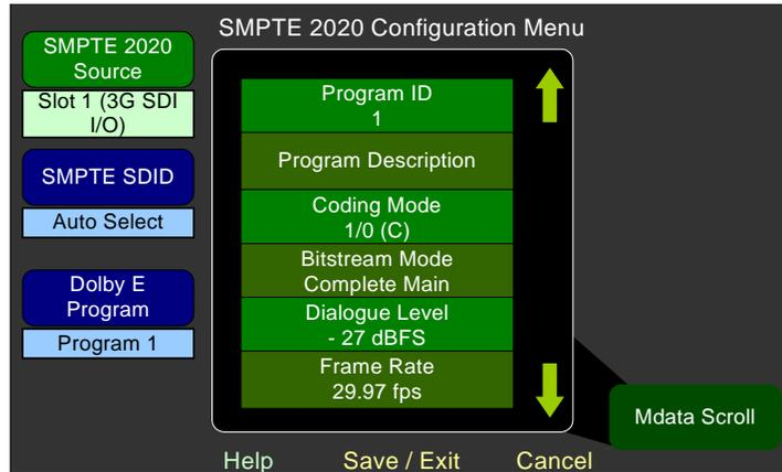
4. Rotate the **SMPTE 2020 Source** to select the input card from which the metadata is to be extracted. The possible choices include any of the 3G/HD/SD SDI cards.
