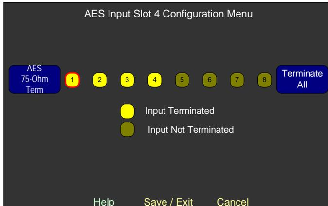
1. To terminate or unterminate all of the AES input pairs on the card in this slot, press **Terminate All**. This is an alternate-action button.
