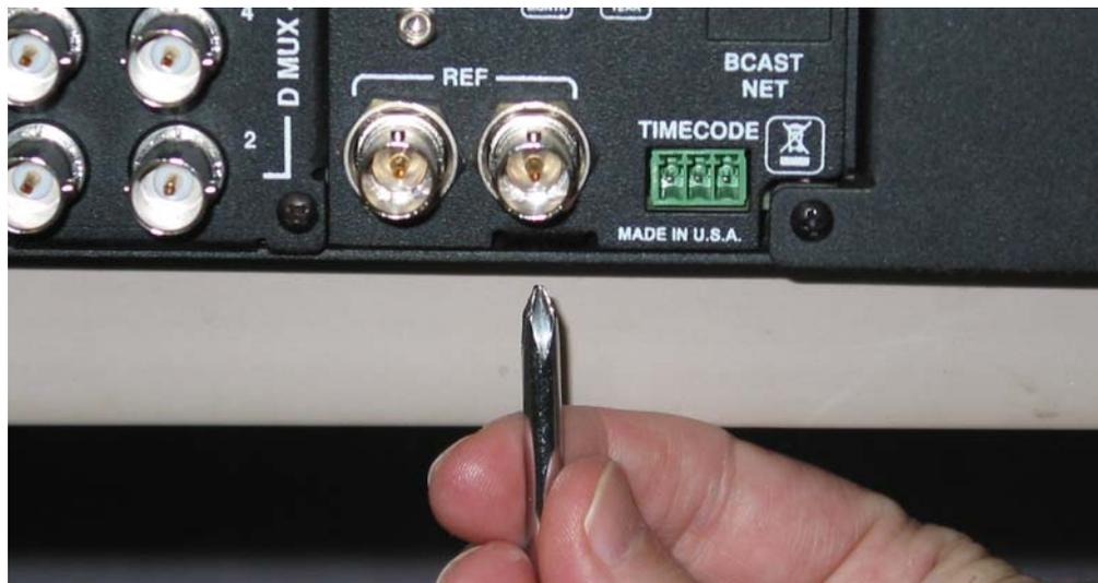
3. Pull the monitor so that it slightly hangs over the edge of the surface on which it is sitting, and remove the screw on the bottom as shown in [Figure 6-10](#) above.
