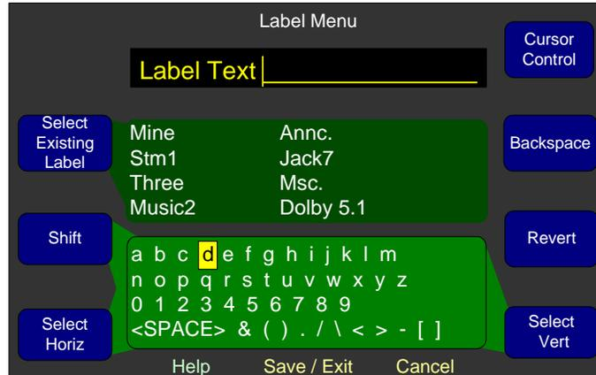
If you see a label in the **Select Existing Label** list that is close to the label you want, rotate the **Select Existing Label** knob until that label is highlighted. Then press the knob to replace the label in the **Label** field with the selected label.
