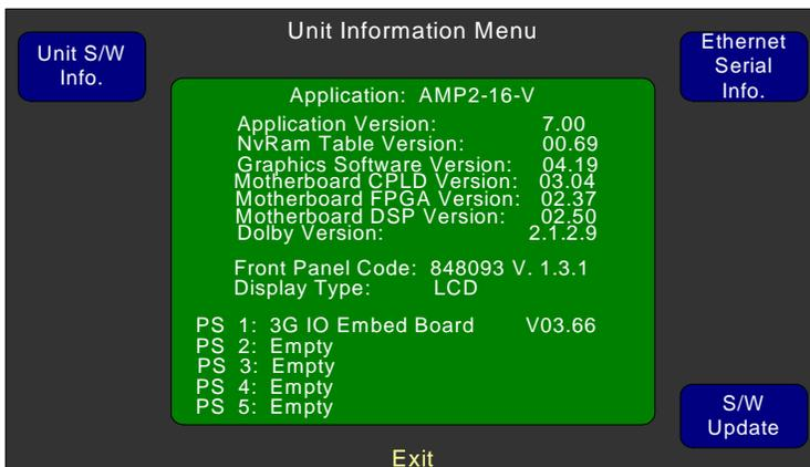
1. The upper part of the screen contains the version numbers of the system software.
