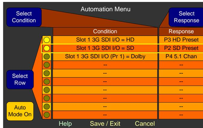
This menu shows ten **Condition/Response** lines that you can individually enable or disable. Each line automatically enables when either a **Condition** or a **Response** is selected. Lines that do not have both a **Condition** and a **Response** are automatically deleted when you exit the menu. The priority of each **Condition/Response** is determined by its position in the list: The higher the position, the higher the priority.
