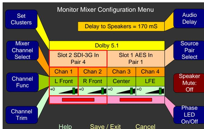
1. Use the **Mixer Channel Select** to scroll to the channel pair where you want the output signals to be displayed.
