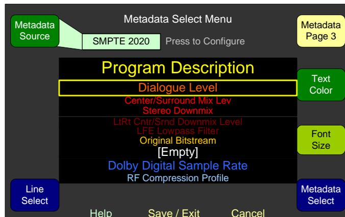
8. Rotate the **Line Select** knob to scroll the highlight up or down among the lines of text to select the one you want to modify.
