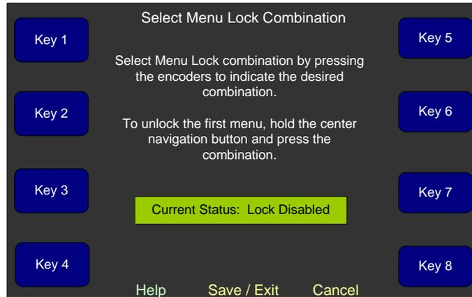
To unlock the menu screen, hold the **Menu** button down (from the **Main Screen**). Then press only the combination buttons (in any order) and no others. Release the **Menu** button and the **Configuration Selection Menu** will appear.
