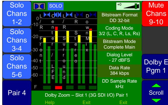
**Note:** The solo and mute keys on the **Dolby Zoom** screen are automatically configured to allow you to easily isolate and listen to the audio of any channel or channels. With the twist of a knob, these hot keys can be converted from solos to mutes. They are automatically labeled according to the Dolby metadata, as are the meter pairs.
