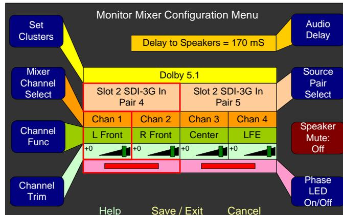
1. Rotate the **Mixer Channel Select** knob to select the channel pair to manipulate.
