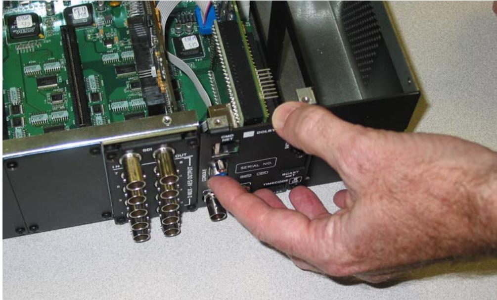
16. Replace the rear panel as shown in [Figure 6–21](#) above.
