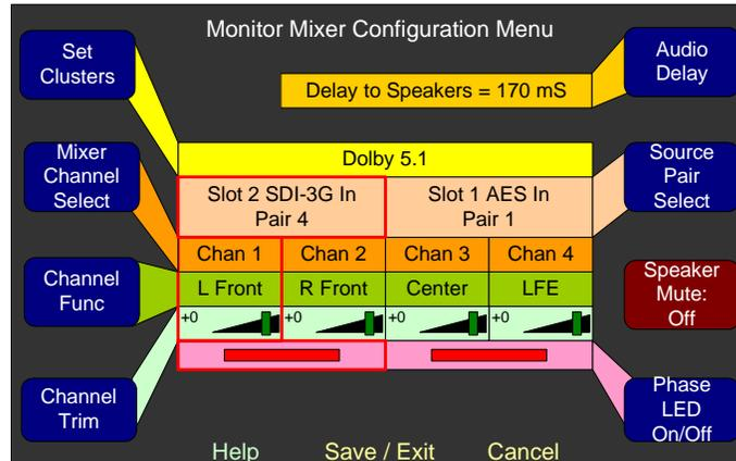
1. Press the **Audio Delay** control to turn on the delay feature.
