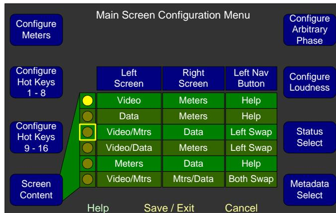
3. When the **Main Screen Configuration Menu** appears, rotate the **Screen Content** knob to select one of the six available arrangements for the left and right screens (shown in [Figure 1-8](#) above). Rotating the knob moves the highlight box; pressing the knob makes the selection. (In these cases, the left navigation button becomes the SWAP button.)
