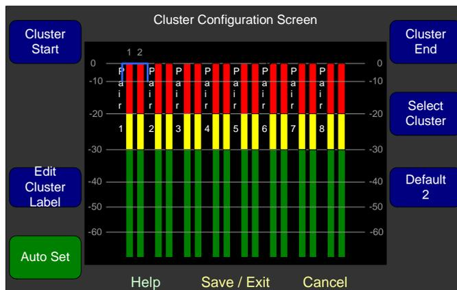
2. Press the **Auto Set** control to automatically adjust the cluster arrangements to match the **Channel Function** settings made in the **Monitor Mixer Configuration Menu**.
