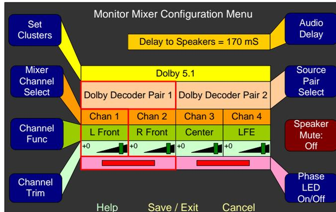
4. Use the **Mixer Channel Select** control to select the channel pair that you want the first decoded Dolby pair to reside on.
