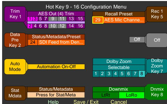
1. Turn the control associated with the hot key you want to be used to quickly recall a preset that the long bar (not the control label) is highlighted. Press the control until the **Recall Preset** or the **Status/Metadata/Preset** function displays.
