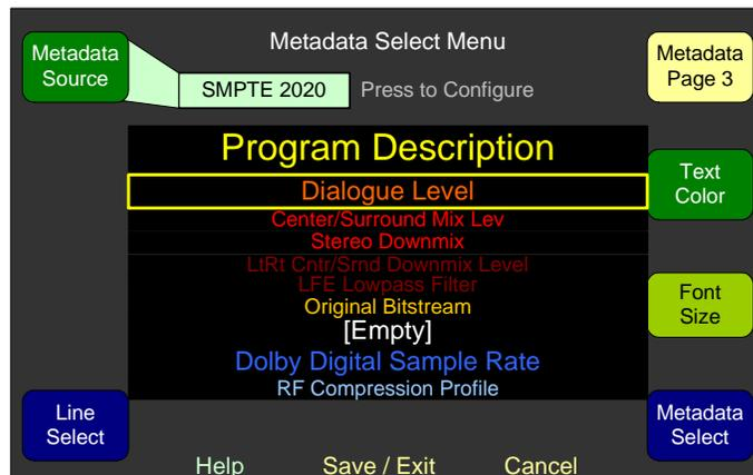
2. Rotate the **Metadata Source** knob to display **SMPTE 2020**, rather than **Dolby Decoder**.
