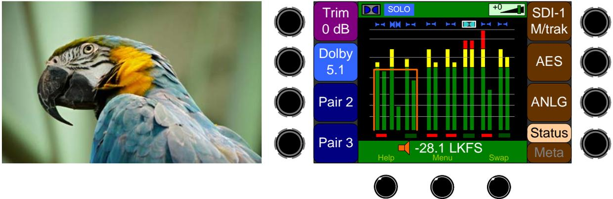
2. Metadata on the left screen and level meters on the right screen (Figure 4–3 below).
