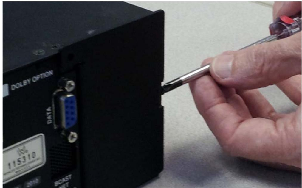
2. Remove the screws on the blank cover plate and remove the cover plate.
