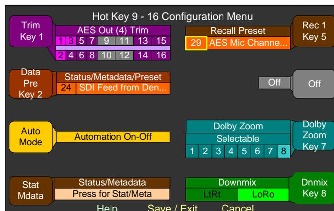
1. Turn the control associated with the hot key you want **Dolby Zoom** to be on so that the long bar (not the control label) is
