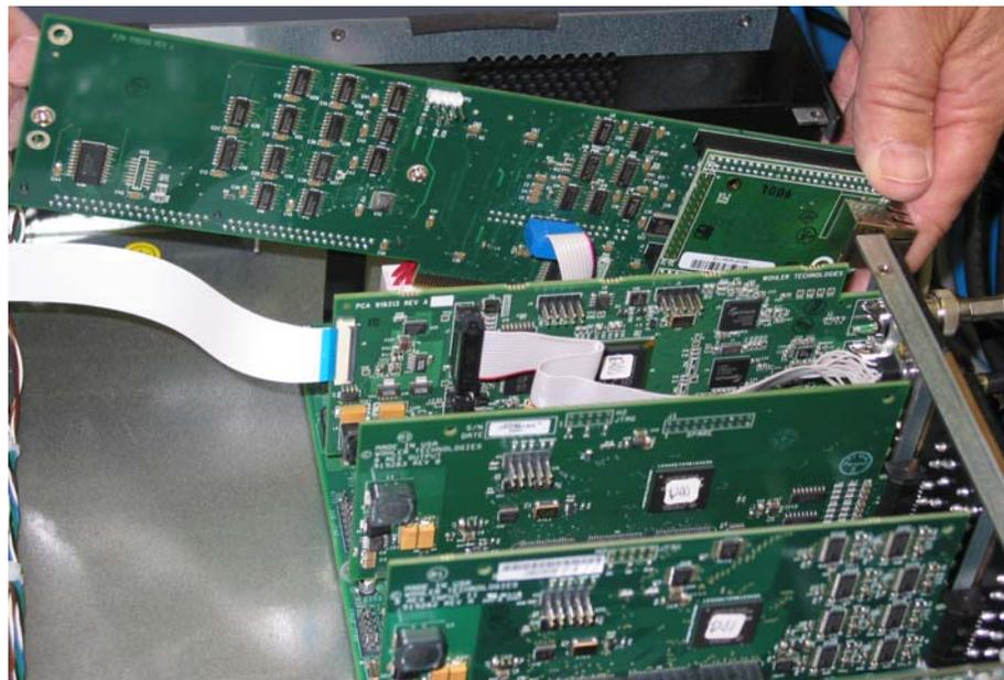
14. Firmly press the system control board back into its slot so that it is securely connected as shown in [Figure 6-20](#). Generally, this board does not snap in.
