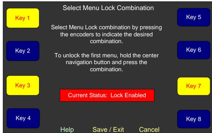
1. Instructions are located on the screen. Simply press the knobs to form an unlocking combination. In Figure 3–27 above, the combination is 1-3-7. Make sure you remember the combination you set!
