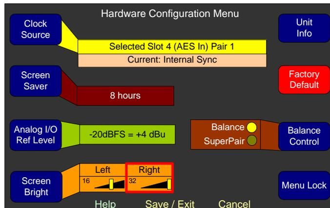
1. Turn the **Clock Source** knob to select the preferred clock and press it. This control will always display the current sync source in the lower rectangle. If the selected source and the current source
