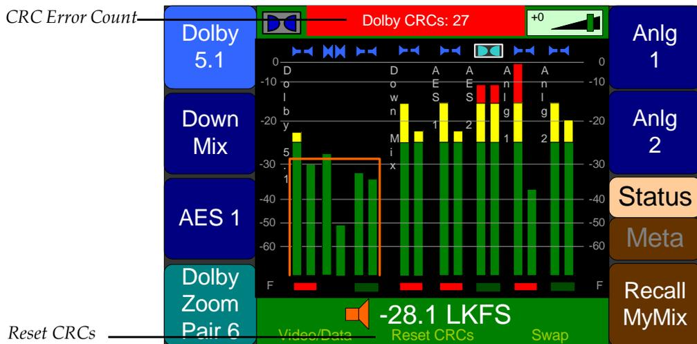
After a few seconds, the red bar turns yellow and will remain until you reset it. Note that when a CRC error first appears, the **Menu** button becomes the **Reset CRCs** button.
