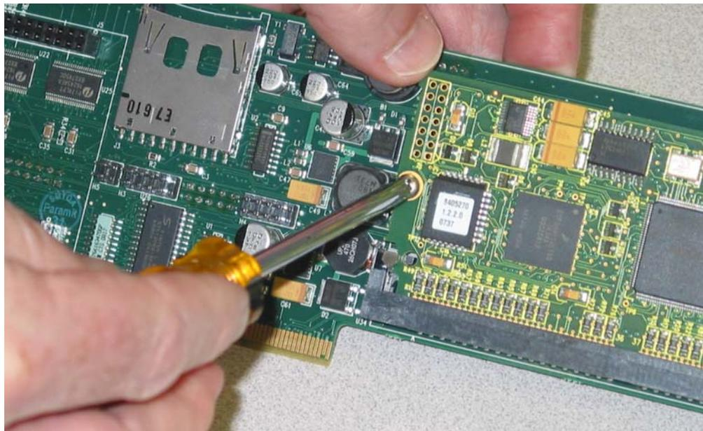
12. Adjust (if needed) and tighten the first standoff screw on the opposite side of the system control board, and then attach another screw on top of the standoff as shown in [Figure 6–18](#) above.
