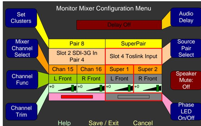
1. Rotate the **Mixer Channel Select** to select the 9th channel pair, the SuperPair.
