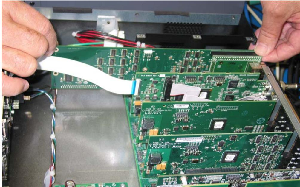
7. Gently tilt the system board out of its slot and remove it from the monitor as shown in [Figure 6-13](#) above.
