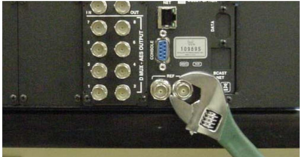
4. Using the wrench, remove the nuts and washers from the **REF** connectors as shown in [Figure 6-11](#) above.
