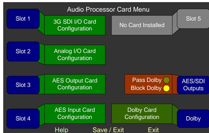
1. Press the control associated with the slot that contains the card you want to adjust ([Figure 3–24](#) above). You may also configure the optional Dolby decoder card.
