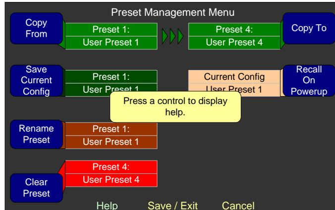
You can display help for any individual knob or button. For example, press the **Help** button on any screen and then press one of the menu/screen controls to display help specific to that control. See [Figure 1-4](#) below.
