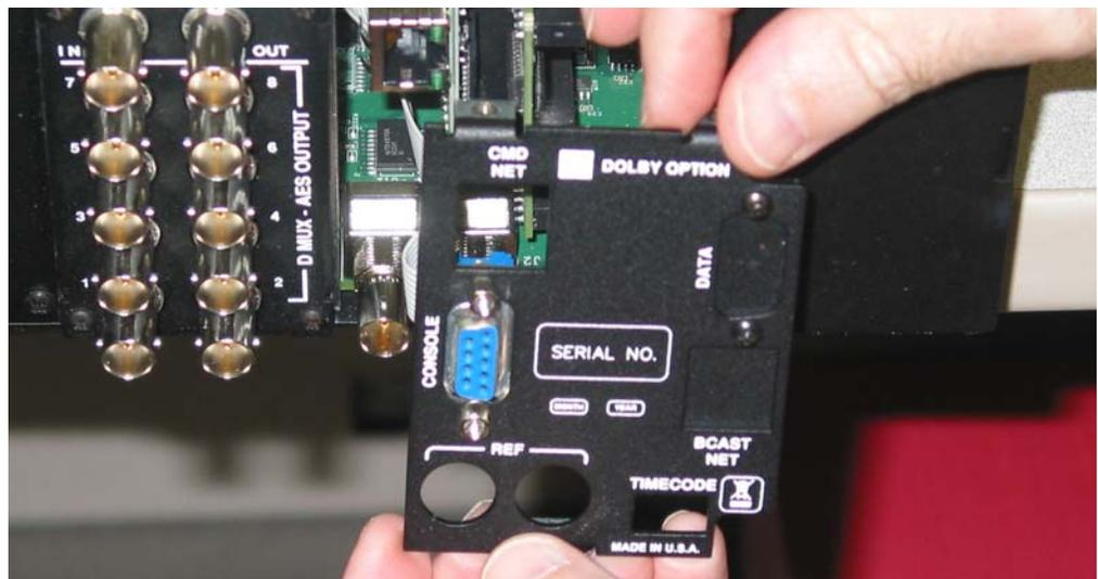
5. Remove the rear panel adaptor for the system control board as shown in [Figure 6-12](#) above.
