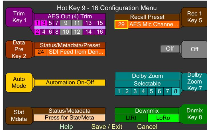
1. Turn the control associated with the hot key you want the downmix to be on so that the long bar (not the control label) is highlighted. Press the control until the purple **AES** or **Analog Output Trim** function displays. If there are multiple output cards, note that the card slot number is shown in parenthesis.
