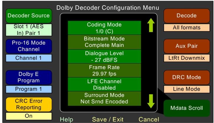
3. Rotate the **Decoder Source** knob to select the source for the Dolby D/E/DD+ Card. The choices include all available AES input pairs, all available SDI de-embedded pairs, and **Dolby Zoom Select**.
