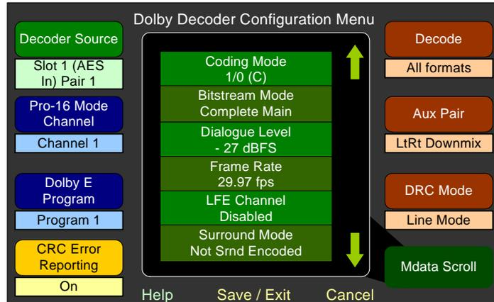
1. Turn the **Decoder Source** control to the AES or SDI channel pair that contains the Dolby bitstream to be decoded.
