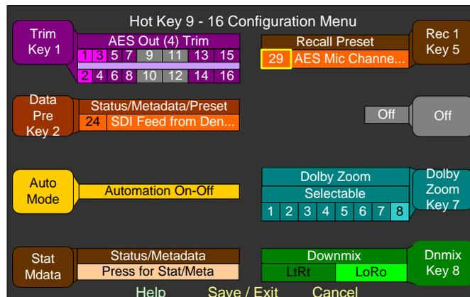
1. Turn the knob associated with the hot key you want the downmix to be on, so that the long bar (not the control label) is highlighted. Press the knob until the green **Downmix** function displays.
