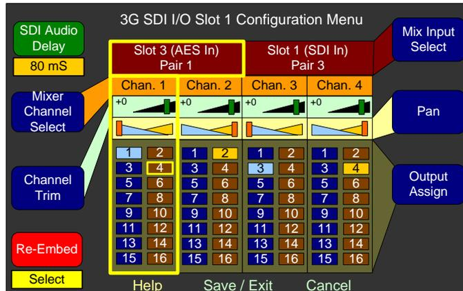
1. Press the **Audio Delay** control to turn on the delay feature. Note that using the **Re-Embed:Select** setting, you can also delay the audio embedded in the reclocked output, which may be useful in synchronizing an external video monitor with the audio signals.
