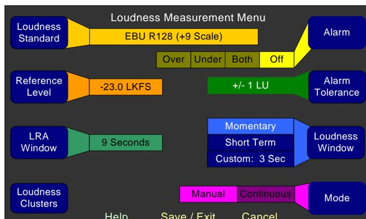
**Important:** In order to calculate loudness accurately, it is crucial that you correctly set the Channel Function for each channel. Depending upon the designated function of each channel, its signal levels will contribute differently to the Loudness calculation. Refer to the [Monitor Mixer Configuration Menu](#) on page 125.
