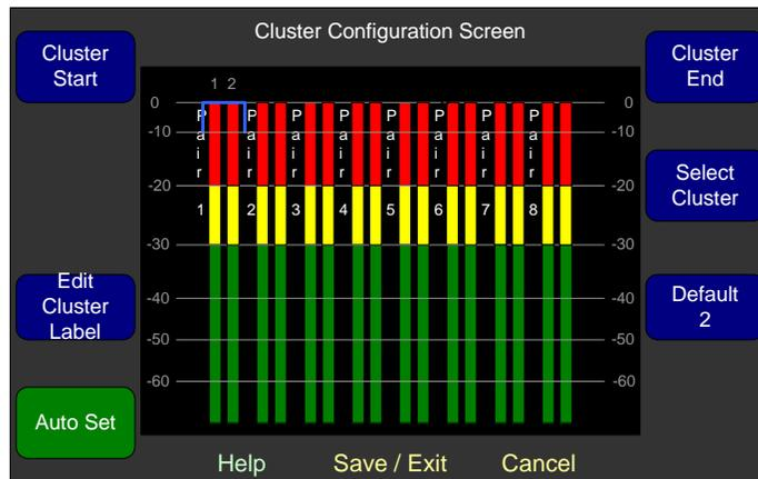
1. If you have already assigned the channel functions in the **Monitor Mixer Configuration Menu**, press the **Auto Set** control and proceed to step 4.
