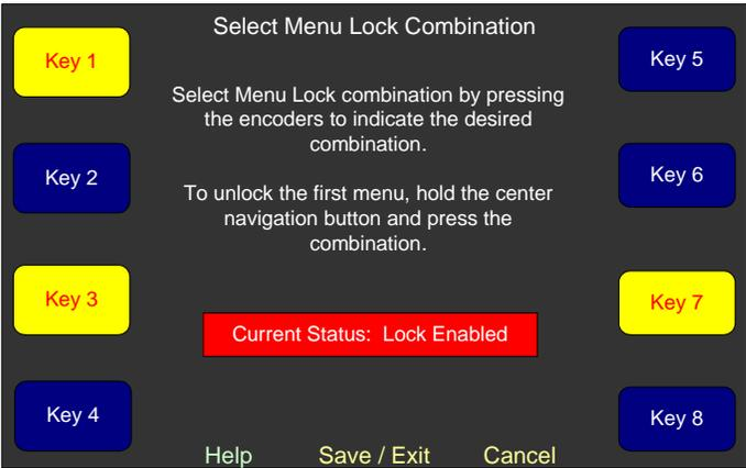
**Keys 1 - 8 - Lock Configuration:** Pressing each control toggles between a bright yellow or a dark blue condition on that control label. The bright yellow labels indicate that the control is part of the lock combination.
