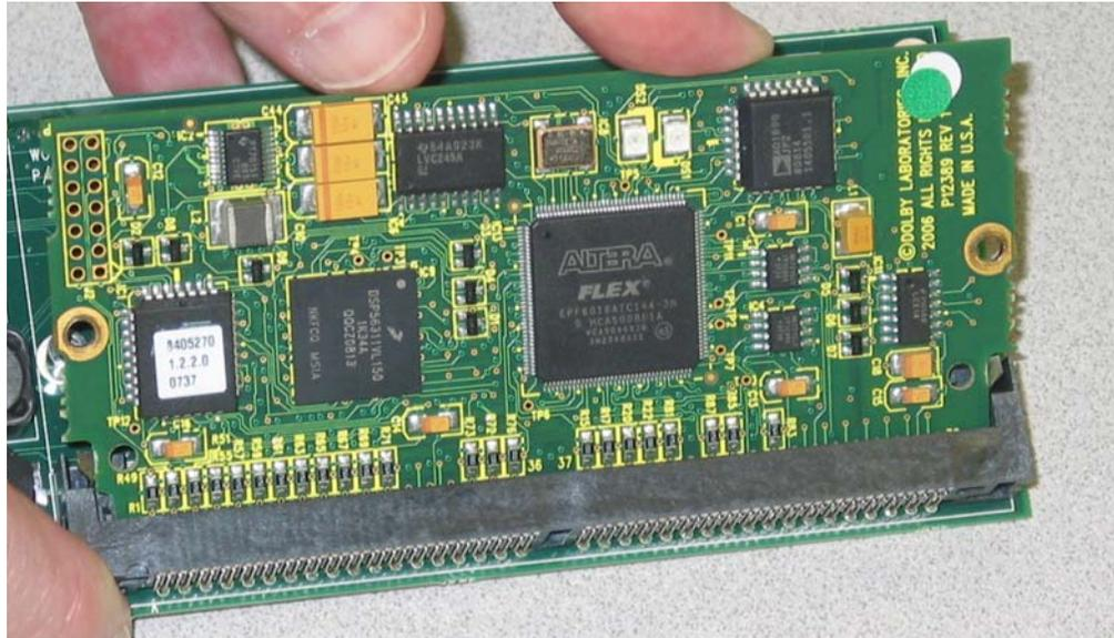
11. Insert the Dolby D/E/DD+ Card into the slot as shown in [Figure 6–17](#) above.
