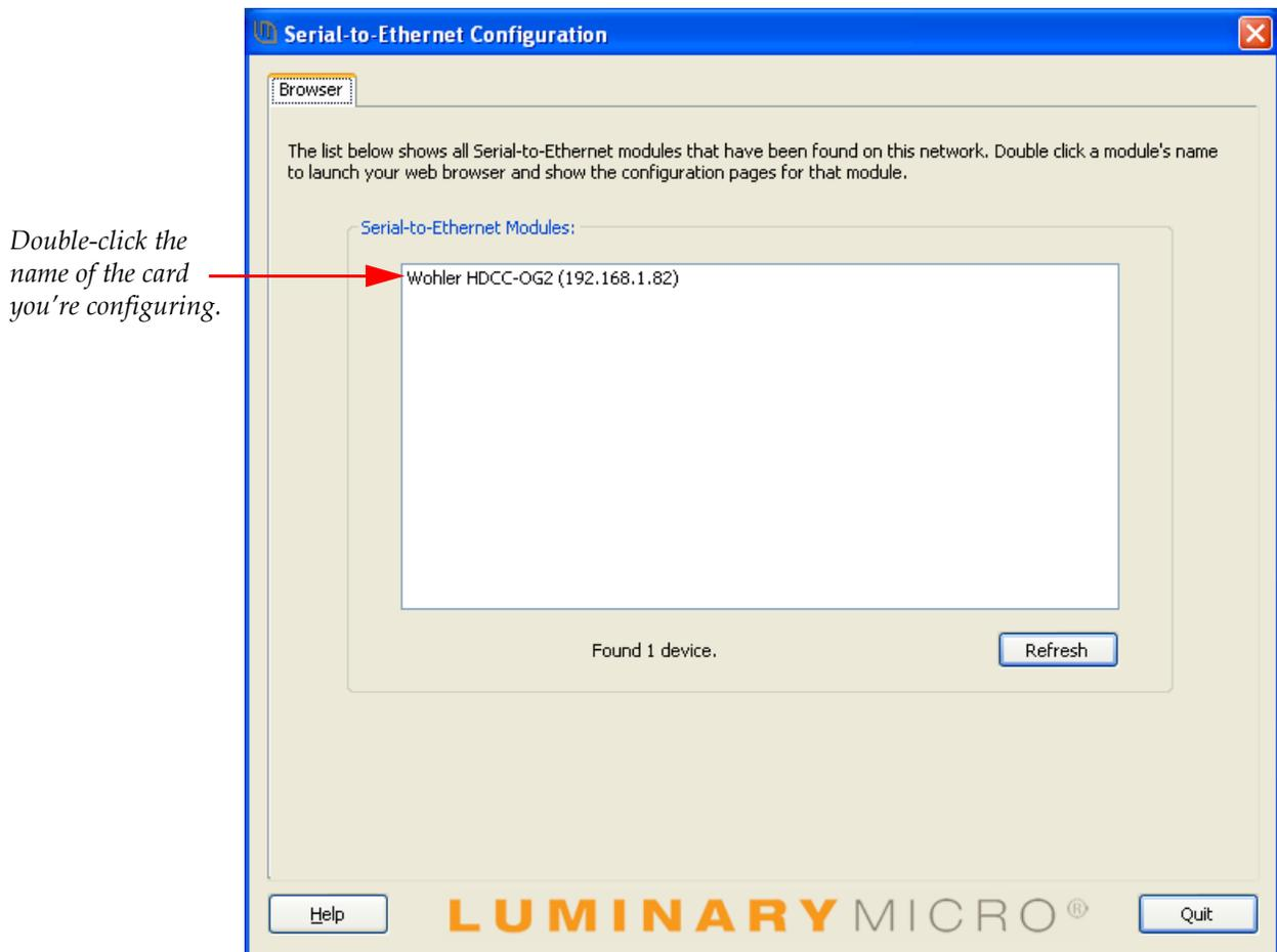
3. Double-click on the HDCC card name as shown in the **Serial-to-Ethernet Modules** pane in [Figure 2-9](#) above. This will take you to [HDCC Configuration](#) below.
