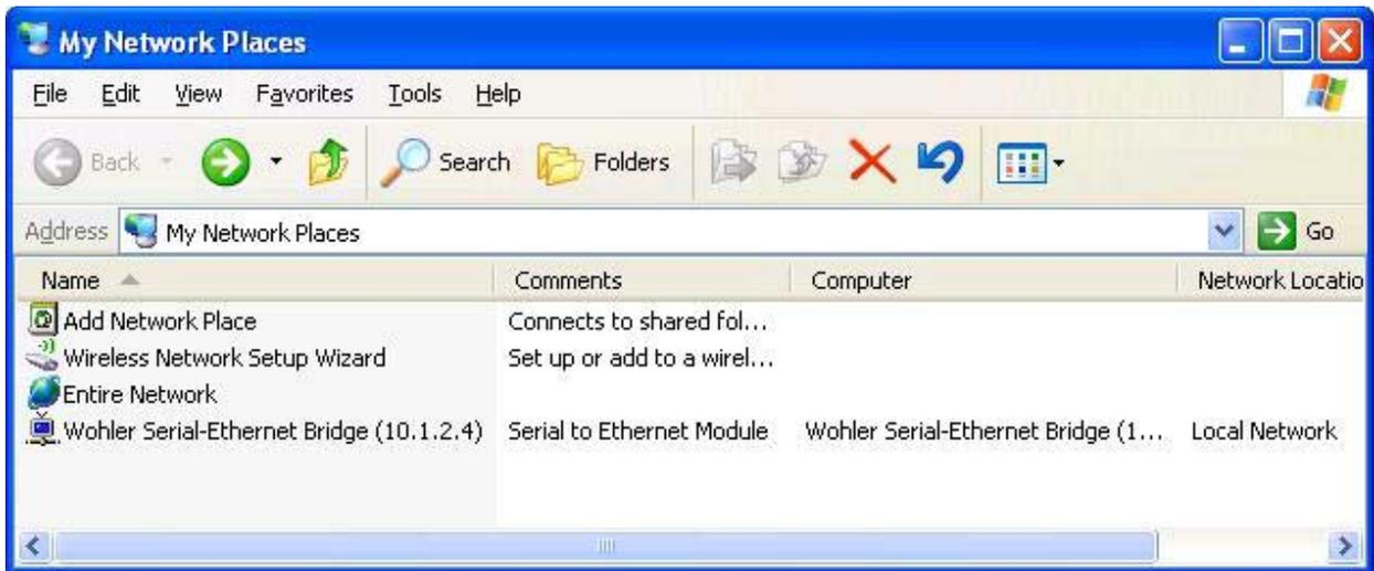
Double-clicking on the Wohler Serial-Ethernet Bridge (see [Figure 2-2](#) above) will take you the card's configuration page where you can set a static IP address, if desired. Proceed to [HDCC Configuration](#) on page 16.
