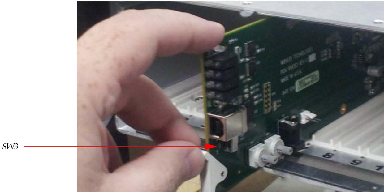
**Note:** Ensure that SW3 is in the **off** position. Refer to [Accessing the Terminal via the USB Port \(Front of Card\)](#) on page 33 for more information.
