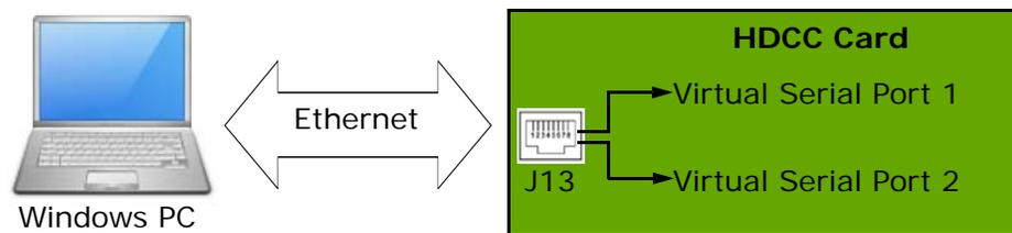
[Figure 2-1](#) above provides a function overview of the virtual serial port configuration. You can use third party software (link provided below) to create a virtual serial port which will transfer serial data to and from the HDCC over Ethernet. From the PC user's perspective, the virtual serial ports are indistinguishable from the hardware serial ports.
