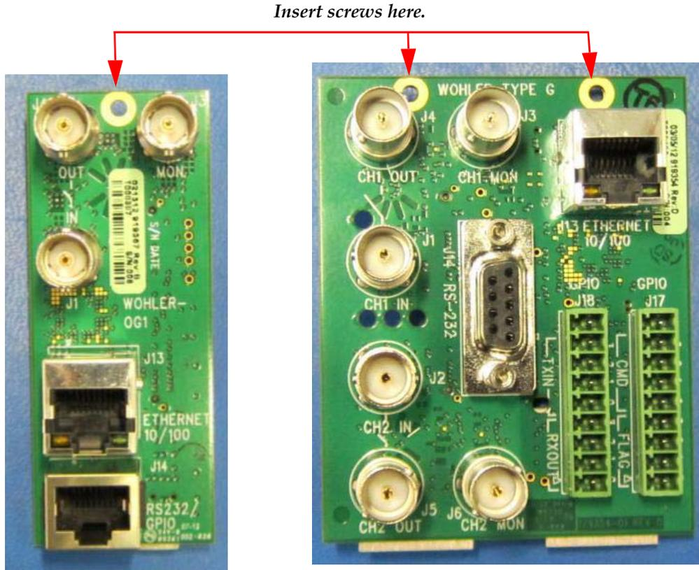
4. After you have inserted the screws into the rear panel, place the rubber washers on the screws. Refer to [Figure 1-2](#) on page 5.
