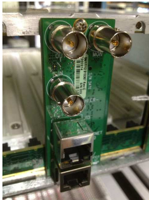
Figure 2-2 Rear Panel Installed
