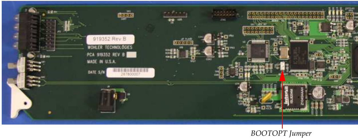
Figure 6–2 BOOTOPT Jumper Location
