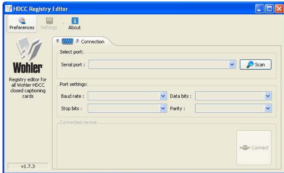
3. On the **Connection** tab, open the drop down list for the **Serial port** and select the serial port that corresponds to your USB port.
