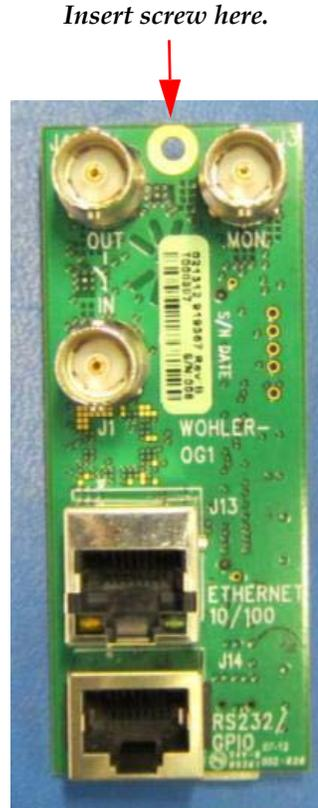
4. After you have inserted the screw into the OG1 Rear Panel, place the O-ring on the screw. .
