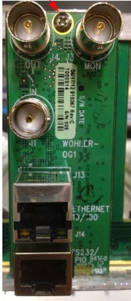
4. After you have inserted the screw into the OG Rear Panel, place the O-ring on the screw. The O-ring will keep the screw from falling out during installation.
