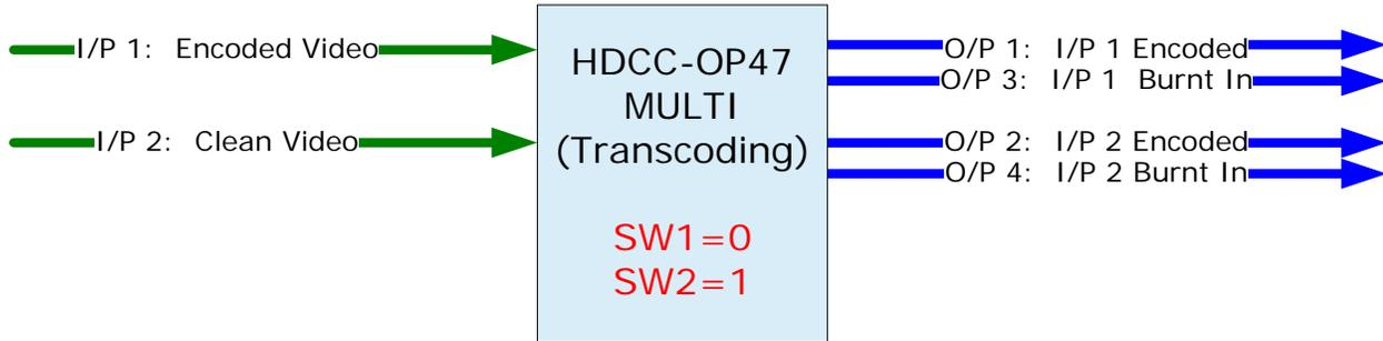
1. Connect the encoded video signal to I/P 1.
