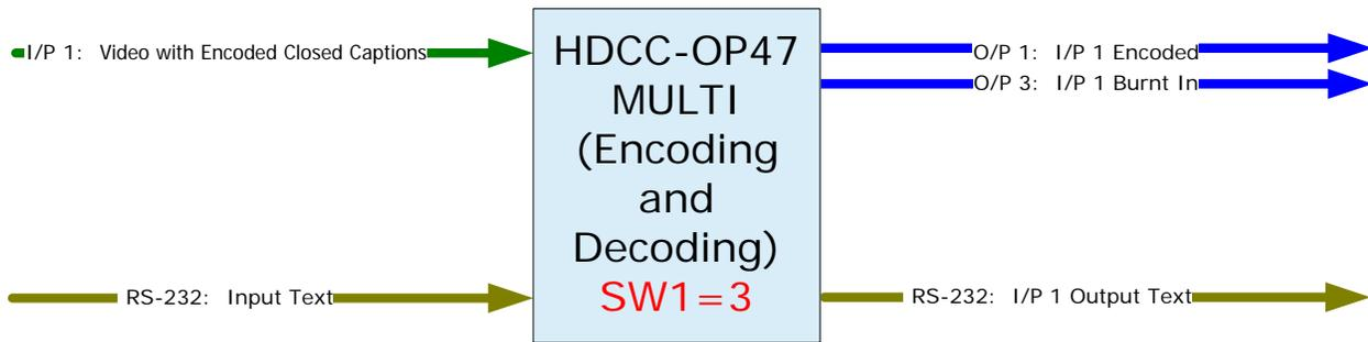
**Example:** This simple example demonstrates the encoding and the decoding features.
