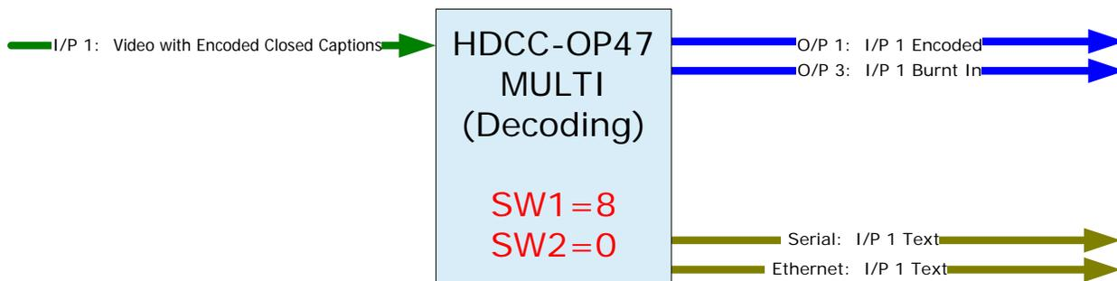
**Example:** This simple example demonstrates the decoding feature.
