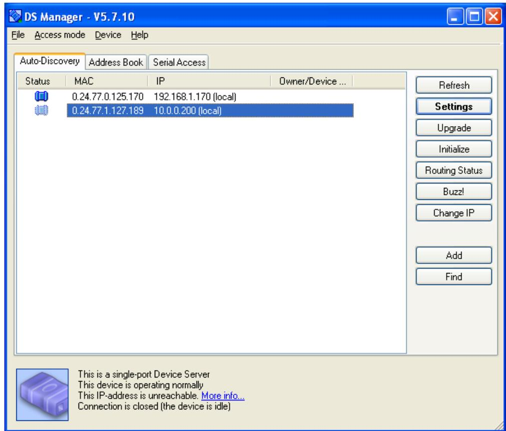
Note that the color under the **Status** column shows IP 10.0.0.200 disabled (i.e., this card is currently not accessible to the network). The card with IP 192.168.1.170 is an existing HDCC on the network.
