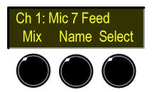
To mix the selected channel position, press the Mix soft key. The mix menu appears:
