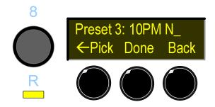
Turn the encoder to select the character indicated by the cursor. Press the encoder to select the character and move the cursor to the next position. Use the **Back** soft key to correct any errors. Up to 10 characters may be entered. When finished, press the **Done** soft key. The front panel display will return to normal.
