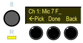
Turn the encoder to select the character indicated by the cursor. Press the encoder to select the character and move the cursor to the next position. Use the **Back** soft key to correct any errors. Up to 10 characters may be entered. When finished, press the **Done** soft key. The front panel display will return to normal.
