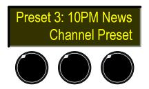
To make changes to the preset, press the **Preset** soft key. The LED beneath each rotary encoder will blink yellow to indicate that they are now to be used in conjunction with the display menu and the display will indicate that one of the rotary encoders must be pressed:
