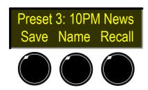
**To recall the selected preset**, press the **Recall** soft key. The preset is recalled and the display returns to normal, showing the number and name of the recalled preset. The 8 LEDs return to their normal function of displaying audio presence.
