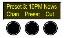
To make changes to a channel, press the **Chan**nel soft key. The LED beneath each rotary encoder will blink yellow to indicate that they are now to be used in conjunction with the display menu and the display will indicate that one of the rotary encoders must be turned:
