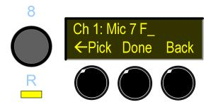
Turn the encoder to select the character indicated by the cursor. Press the encoder to select the character and move the cursor to the next position. Use the **Back**space soft key to correct any errors. Up to 10 characters may be entered. When finished, press the **Done** soft key. The front panel display will return to normal.
