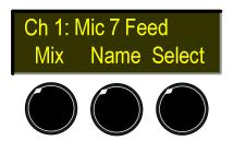
To mix the selected channel position, press the Mix soft key. The mix menu appears with the current selection underlined:
