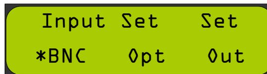
2. Press the **BNC** button (Figure 1-6) to select the audio coming in on the BNC connectors, or press the **Optical** button to select the audio coming in on the optical connectors. Note that as soon as you press one of these buttons, the system will display an asterisk next to it to indicate that this is the selected input.
