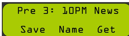
After pressing the **Get** button, the system changes to the recalled preset and the display returns to normal view, displaying the preset you just selected.
