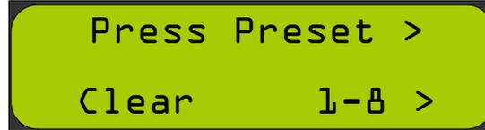
2. Press the **Volume/Mute** knob that corresponds to the preset you want to create. (Each of the eight presets corresponds to each of the eight **Volume/Mute** knobs.) The LED for the selected preset will glow steady yellow and the other LEDs will turn off.
