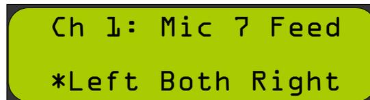
**Note:** By default, all odd-numbered channels are directed to the left speaker, and all even-numbered channels are directed to the right speaker.
