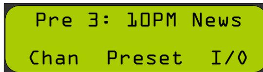
1. To create a new preset, press the **Preset** soft key ([Figure 1-14](#) above). The LEDs will blink yellow to indicate that they now indicate that one of the **Volume/Mute** knobs must be pressed.
