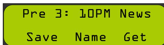
After pressing the **Name** button, the system displays the text entry menu ([Figure 1-18 on page 16](#)) indicating that **Volume/Mute 1** knob has been temporarily re-purposed to select text. **LED 1** will blink yellow at the same rate as the blinking text cursor on the screen.
