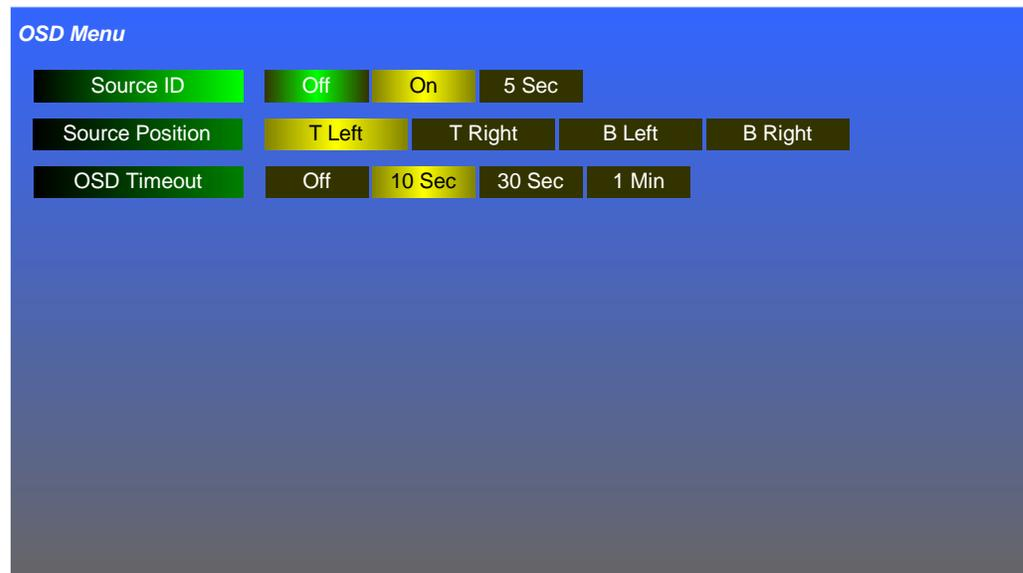
Rotate the **Volume** knob to highlight the item to be adjusted, and then press to enter it. Again rotate the **Volume** knob to the option selection and press to choose it:
