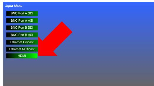
2. Press the **Input** button to display the **Input Menu** and then turn the **Volume** knob to move the selector to **HDMI**. Press the **Volume** knob once to select **HDMI**.
