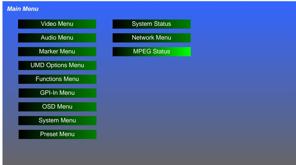
Rotate the **Volume** knob to highlight the menu you want to access and then press to enter it. In this or any menu, press the **Menu/Back** button to back out of the menu or the particular selection within that menu. The menus are described on the following pages.
