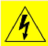
The symbol to the left warns of electric shock hazard inside the unit. Disconnect the power cord before removing access panels when installing upgrades. Only qualified service personnel are to operate the equipment with covers removed, and are to exercise caution to avoid personal injury or damage to the equipment from overheating.
