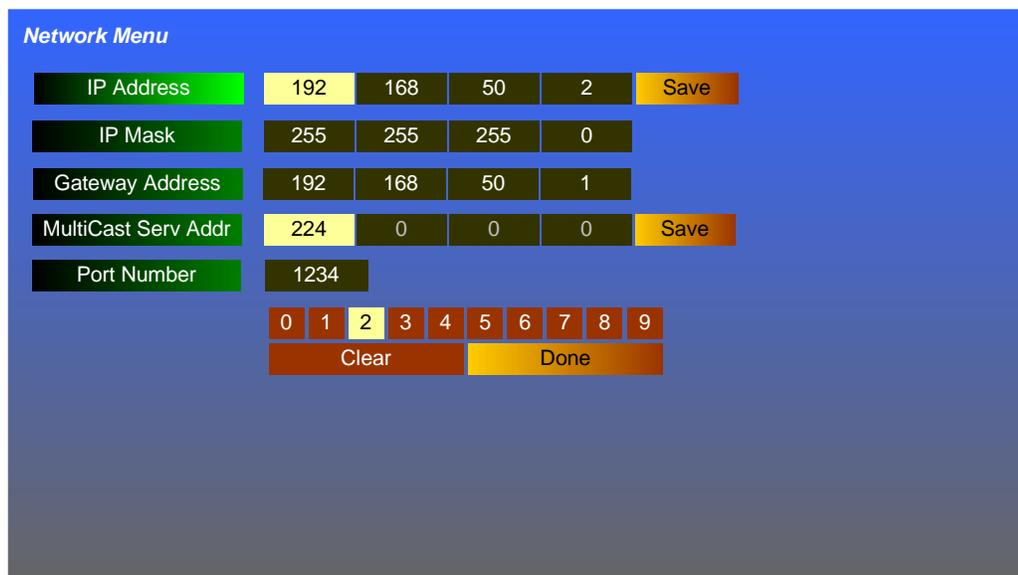
Rotate the **Volume** knob to highlight the item to be adjusted, and then press to enter it. Again rotate the **Volume** knob to the item you need to change and press to replace it. A number in the keypad below will then be highlighted. Rotate and press to select the new numeric entry. Use **Clear** to start over and **Done** when finished. The changeable fields are as follows:
