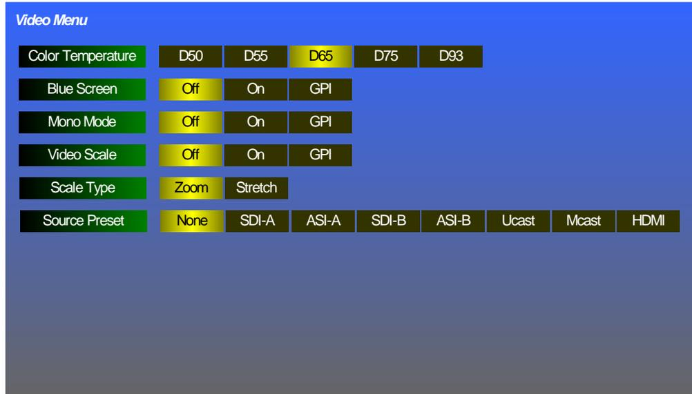
Rotate the **Volume** knob to highlight the item to be adjusted, and then press to enter it. Again rotate the **Volume** knob to the option selection and press to choose it:
