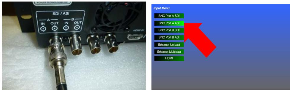
3. When you see **ASI -A:TSSync** on the screen, the signal has been recognized and the lowest-numbered viewable program will be displayed.
