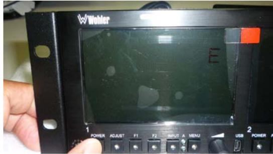
5. For 30 seconds, the **Power** indicators should flash. Then the screens should show a progress bar, followed by some white flashes and a splash screen showing the MPEG Series product line. The start up process takes just over a minute. When the start up process is complete, you should see a screen similar to the following:
