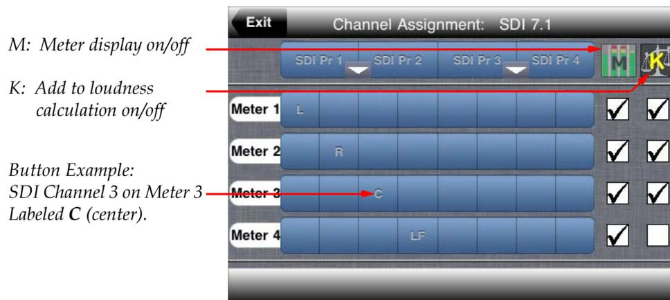
4. To assign a channel to a meter, simply touch the blue button that represents the intersection of both the channel and the meter you want to assign the channel to. In the example in [Figure 2-12](#) on the previous page, Channel 1 is assigned to **Meter 1** as **L**; Channel 2 is assigned to **Meter 2** as **R**; Channel 3 is assigned to **Meter 3** as **C**, and so on.
