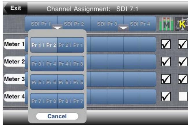
7. Now for each meter, touch the blue boxes to display the channel type list as shown in [Figure 2-15](#) below.
