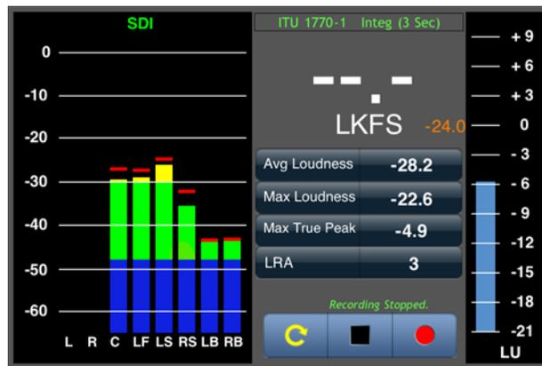
Note the LU meter scale indicator at the bottom right hand corner of the screen. Pandora has one ATSC, and two EBU scale ranges. (Zero LU is equal to the **Reference Level**.)
