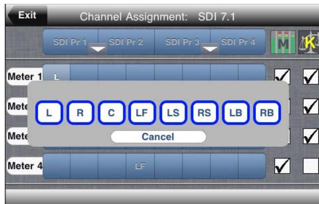
8. Touch the channel type for this meter ([Figure 2-15 on page 21](#)):
