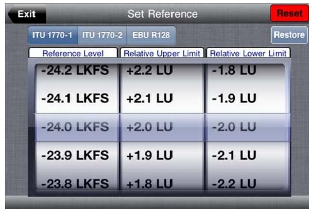
**Note:** The ITU 1770 settings include ITU-R BS.1771 and ITU-R BS.1864 (-24 LKFS) international standards which are called out by various regional standards such as ATSC A/85 and ARIB TR-B32. LRA is included as an additional loudness measurement for both ITU configurations, even though it is not required by any BS.1770 version.
