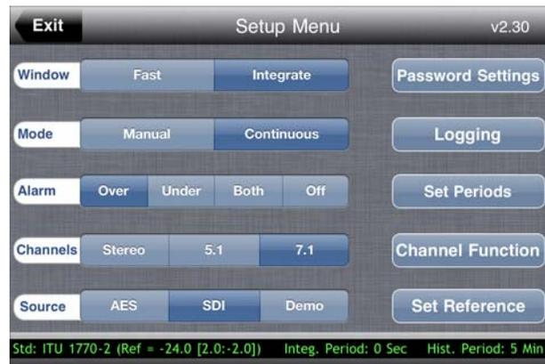
1. From the **Setup Menu**, touch **Logging**. The **Logging** menu displays today's date and the number of logs found for the day (Figure 3–3 below). In the example below July 16th no logs are available.
