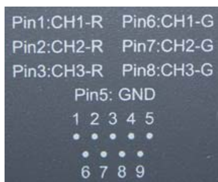
Figure 1–4 Rear Panel DB9 Connector Pin Out
