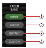
Allows you to select which fader bank is displayed in the channel strip area (→page 11).
