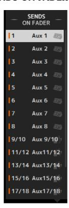
Allows you to use the channel strip area temporarily to adjust SEND LEVEL and SEND ON for the desired buses.
