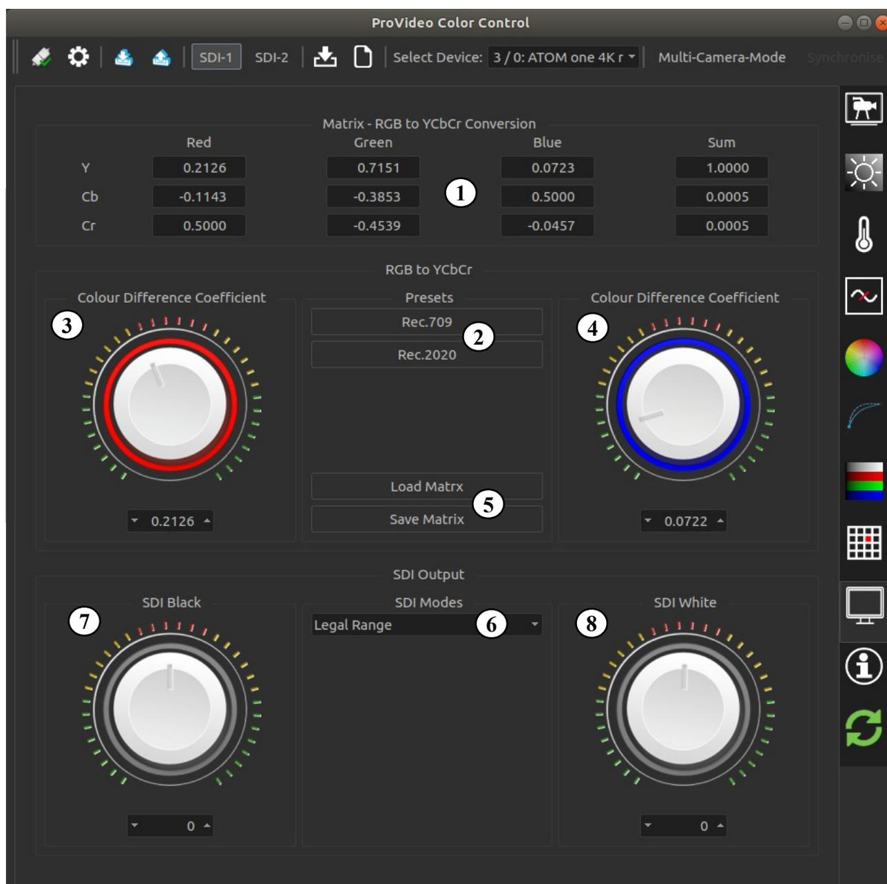
The screenshot displays the ProVideo Color Control interface. The main section is titled "Matrix - RGB to YCbCr Conversion" and contains a table of conversion coefficients:
