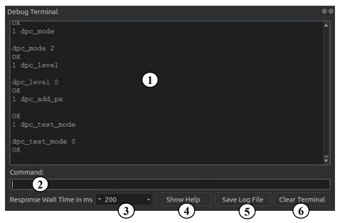
The Debug Terminal shows all commands which are send by the GUI. It can also be used to manually send commands to the device.
