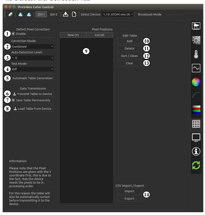
Enable the defect pixel correction module.
