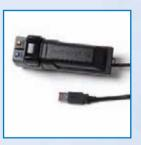
The New RAT II USB Hand controller can be used with WinPlus X-Lite. A Rocker scroll control with Forward / Reverse control and centre stop. Previous and next item selection via two-button control. One button press to select top of runorder. Simple plug and play technology, with all drivers supplied within the WinPlus software.
