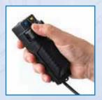
The Autoscript RAT2 i-Plus plugs directly into Scroll Plus Adaptor via the 30 way connector on the i-Touch/Phone or i-Pad.
