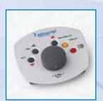
Potless five button deskpad control offers rotary speed control for +WinPlus+ Studio and News. It includes page/bookmark/snapshot next or previous, back to top of script function, blank screen and a programmable function button. Suitable for use on locations or studios. Control Net Enabled.
