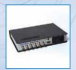
Up to four Opto Hand or Foot controls can be used with the PCIPrompt card using the Smart Combiner box. The box plugs into the 9-way/D connector PCI Prompt card. It has four coax inputs that accept connections from the controllers via their associated coax adapters (see previous section for adapter details). Smart Combi's can be linked via standard 75 ohm coax cable and can be located up to 300 meters from one another.
