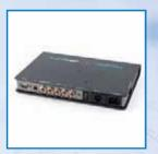
Based on our successful Xbox USB external box solution for prompting, the Xbox Ultra provides enhanced features and capabilities making even more ideal, especially for portable prompting. Just plug into a laptop or PC via the USB interface. The video output is standard composite PAL or NTSC and is compatible with all our on-camera Units. It runs with exactly the same WinPlus versions that run with the PCI Prompt Card, no additional operator training will be required.
