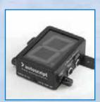
+TallyPlus+ is a unique camera number system. A large LED indicator displays the camera in green (1-9) while in standby, then turns red when the camera is live. Switching from green to red is achieved by a photo electric cell that can be attached to the camera tally light. +TallyPlus+ retro-fits to the whole range of Autoscript TFT's and has the unique feature of a second photo electric cell built into the rear of +TallyPlus+ that docks with cue light on the TFT.
