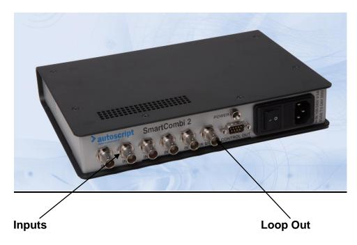
The Smart Combi unit combines four control inputs into one control output. Units can be "daisy chained" together to increase the number of control inputs to control a single Autoscript PCI PromptCard. If more than four remote inputs are required the Smart Combi Boxes can be "daisy chained" together. The realistic limit to the number of Combi Boxes is 7 with this amount there will be no delay. As an example, we have installations using five boxes to give 20 remote inputs.
