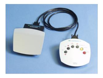
A Six button, desk pad is available. The button functions are: Story Next, Story Back, Toggle Forward/Reverse, Back to Top of Script, Programmable Function, Blank Screen.
