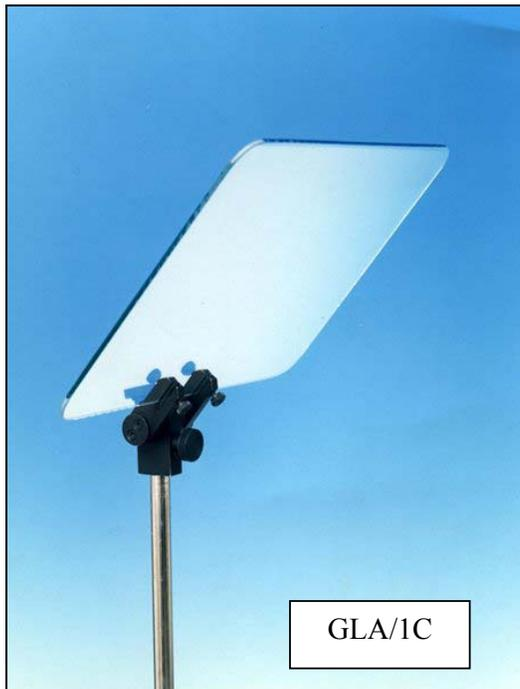
The Glass support is shipped in two pieces the inner rod (F) can be lengthened by screwing both parts together for a standing Speaker or by using only one piece for a sitting speaker, one inner rod is already fitted inside the lower tube (G) This is fitted into Block (H) And tighten thumbscrews.
