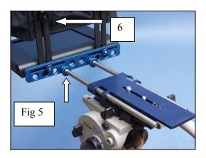
Make sure that the blue knurled nuts (5) are fully undone, away from the stainless "buttons". Drop the Hood/Monitor assembly over the ends of the rods and tighten the knurled nuts. Ensure that the stainless "buttons" are seated in the recesses on the face of the blue cross-mounting bar.
