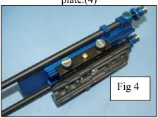
Replace the pan and tilt adaptor plate back on the pan and tilt head.
