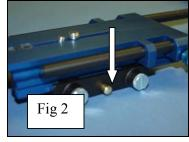
Attach the camera plate to the top of the blue mounting plate with the front of the cameraplate set back about half an inch back from the front. (3)
