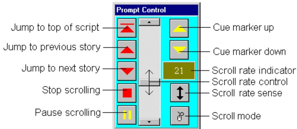
The prompt rate indicator will show negative numbers when scrolling backwards, PAUSED when paused and STOP when the scroll rate is zero. The pause button is a toggle, when it is pressed after pausing, the prompt rate returns to the original setting before pausing had taken place.
