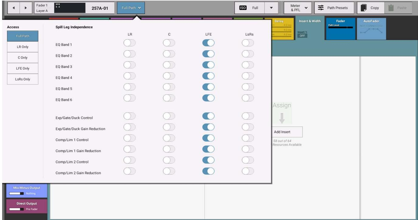
Figure 9 shows the 'LR Only' spill legs on the Inserts page. As this is a Stereo spill leg all the controls that would normally appear for a Stereo Insert including Width are made available. Note: the LsRs spill legs appears with the same parameters controls as shown here for the LR spill legs. The C and LFE spill legs appear in a similar way but without width controls.
