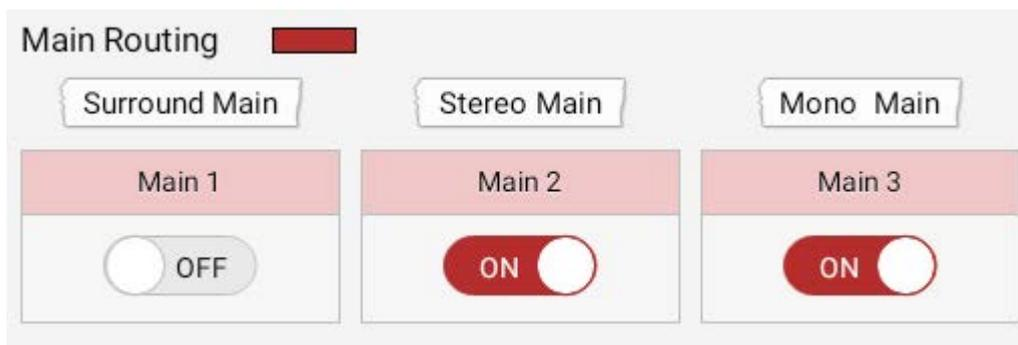
4. If routing to an output (direct or mix minus), tap either **MONO** or **STEREO** to create the desired output for the accessed path.
