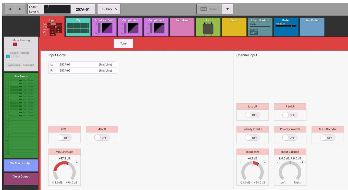
Figure 10 shows the 'C Only' spill leg on the Input page. As this is a Mono spill leg all the controls that would normally appear for a Mono path are made available. The 'LFE' spill leg appears with the same mono parameters controls as shown here for the C spill leg. Note the Mic Gain for this spill leg.
