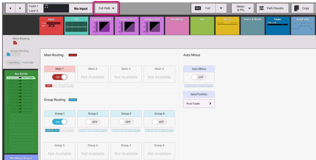
When a partial route to a bus is made, i.e. only some of the spill legs are routed, the routing indicator from the 'Full Path' view shows the Route with the top right hand corner cut off and in addition the routing blocks underneath the 'Full Path' routing switches show which spill legs have been routed. So in Figure 4 Fader1's 5.1 channel has routed just the front LR spill legs to Main 1 and has routed the LR & C spill legs to Group 1.
