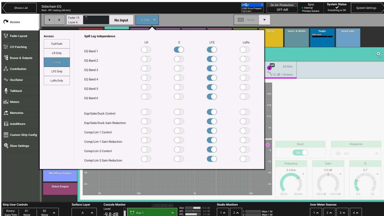
As shown in Figure 4 all the controls for the LFE spill leg are independent, this is by default. The user has just made EQ band 1 independent for the C Only spill leg of this 5.1 channel. Figure 5 on the next page shows the EQ control for Band 1 of the C Only spill leg.
