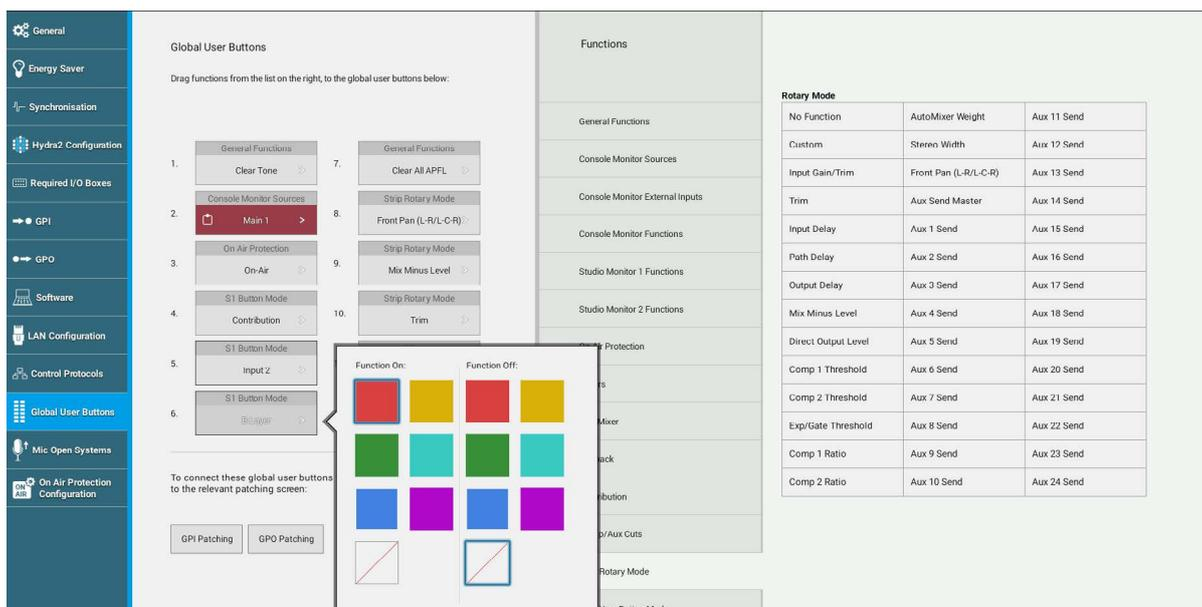
Global User Buttons are setup by dragging and dropping the function onto the required button.
