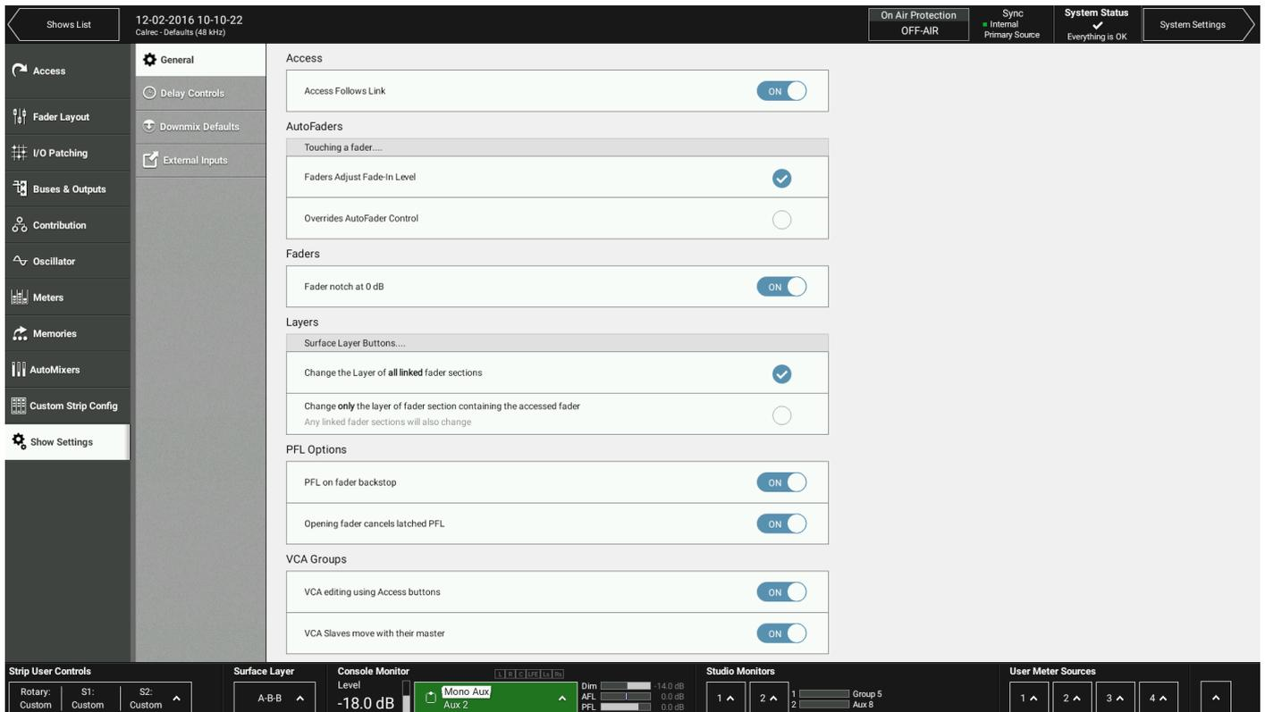
When this option is on, then when the user creates a link across a range of faders by simultaneously pressing two access buttons, the left-most path in the link will be accessed. Using this option eliminates the worry about accessing the right path after the link is created.
