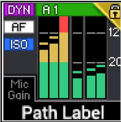
This fader is neither master nor slave. If a path is attached, the level of this fader is the level of the path.
