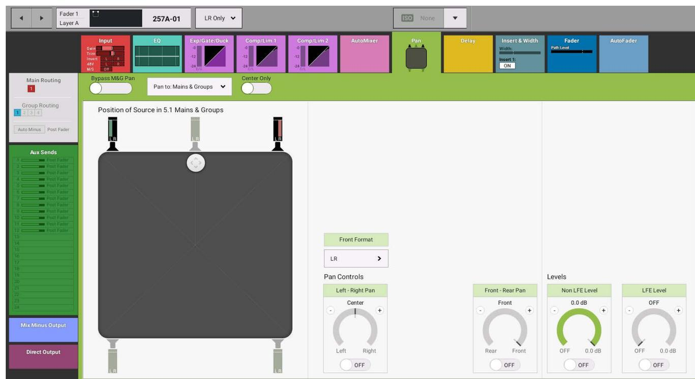
Figure 5 shows the 'LFE Only' spill leg on the Pan page. As this is a Mono spill leg all the controls that would normally appear for a Mono path are made available. Note: the 'C ONLY' spill leg does not allow any panning as it is by definition in the centre of the soundfield.
