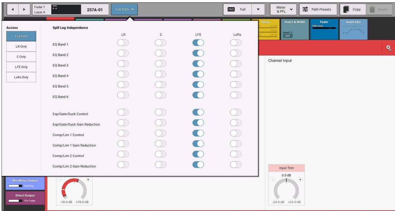
Figure 9 shows the 'LR Only' spill legs on the Input page. As this is a Stereo spill leg all the controls that would normally appear for a Stereo path are made available. The 'LsRs' spill leg appears with the same stereo parameters controls as shown here for the LR spill legs. Note the Mic Gain for this spill leg.
