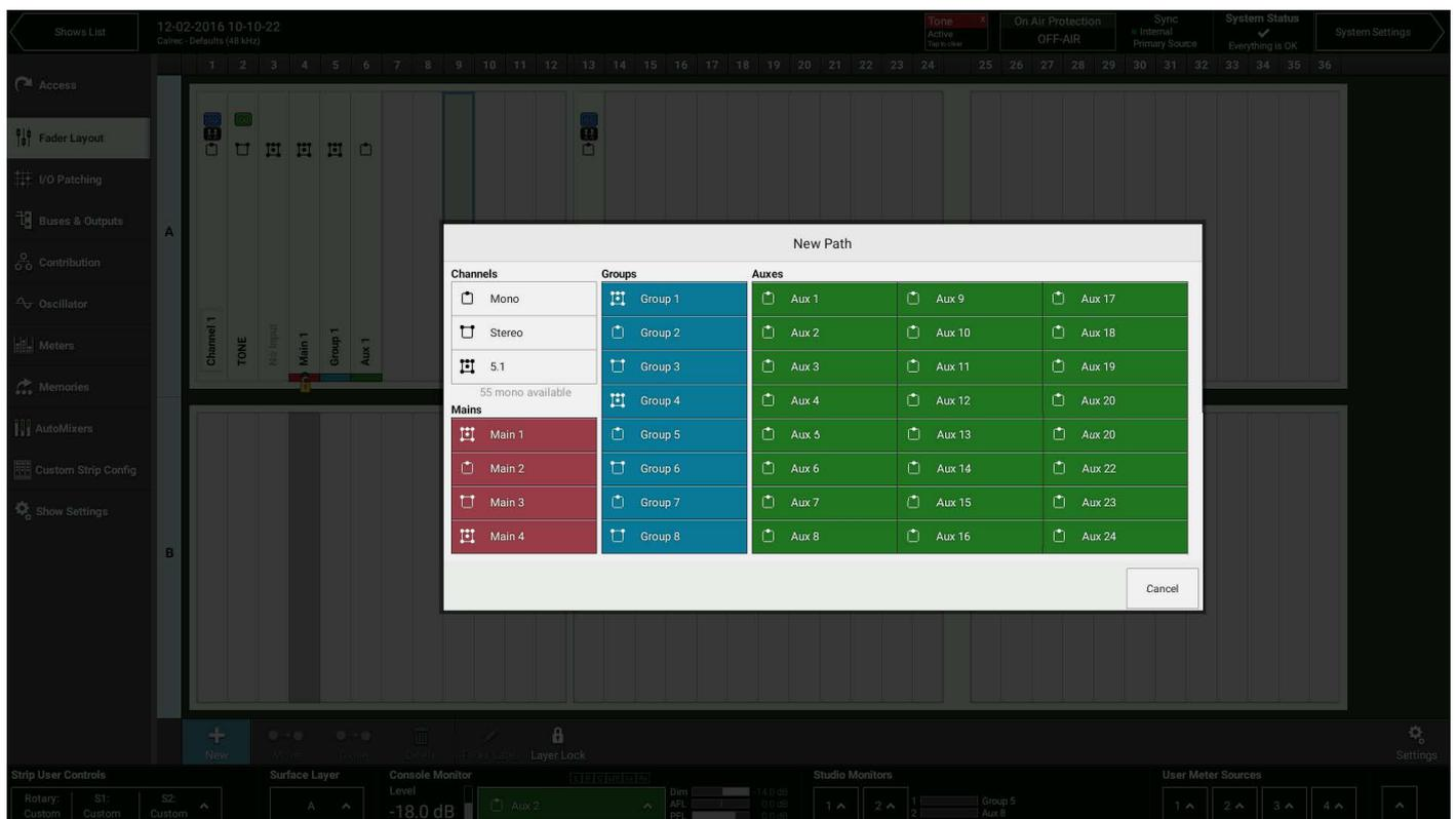
Note: when viewing the access screen, if a fader with no path allocated is accessed, the screen provides a short cut to assign a path and will work in conjunction with linked faders to allocate multiple path at a time.
