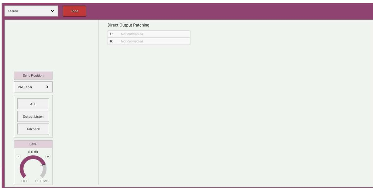
Note: buttons that route tone to audio paths are disabled whilst the console is in On-Air mode, and entering on-Air mode will also clear any tone routing that is active.
