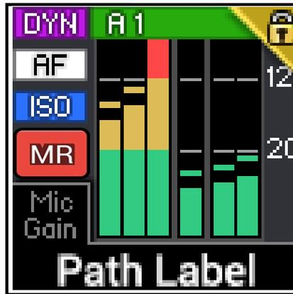
This fader is a primary master. If a path is attached, the path is a direct slave to this master. Push ACCESS to see and alter the level of the slave path.
