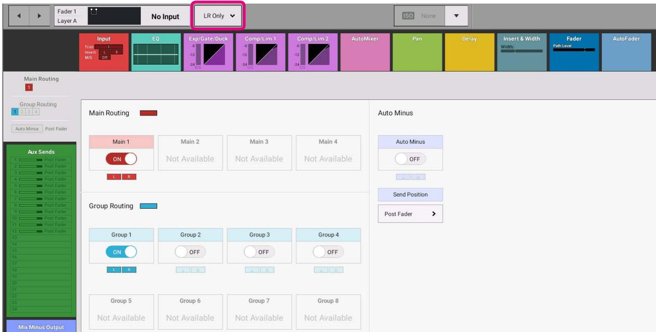
Note: that in Figure 3 the Main 1 and Group 1 routing displays are just showing the L and R indicators underneath the routing switches. Selecting the 'Full Path' button again and this time selecting 'Full Path' returns the routing display back to showing the routing for all the spill legs as shown in Figure 4 below.
