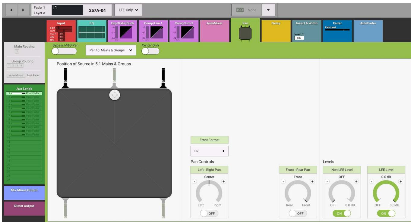
Figure 6 shows the 'Full Path' on the Pan page. As this is the 5.1 Channel it shows no Pan controls available as it is by definition a 5.1 source..
