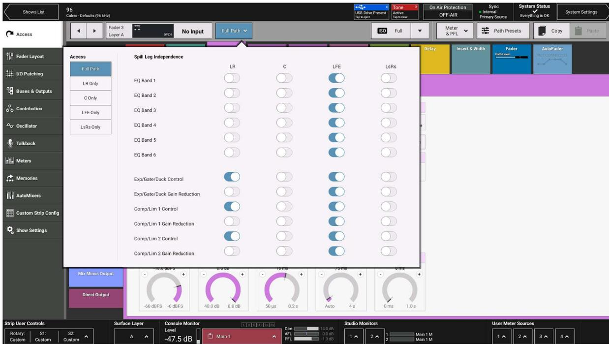
As shown in Figure 13 all the controls for the LFE leg are independent, this is by default. The user has just made the Expander/Gate/Ducker, Comp/Lim1 & Comp/Lim2 controls independent for the LR Only spill legs of this 5.1 channel. Figure 14 shows the Ducker control for LR Only spill leg.
