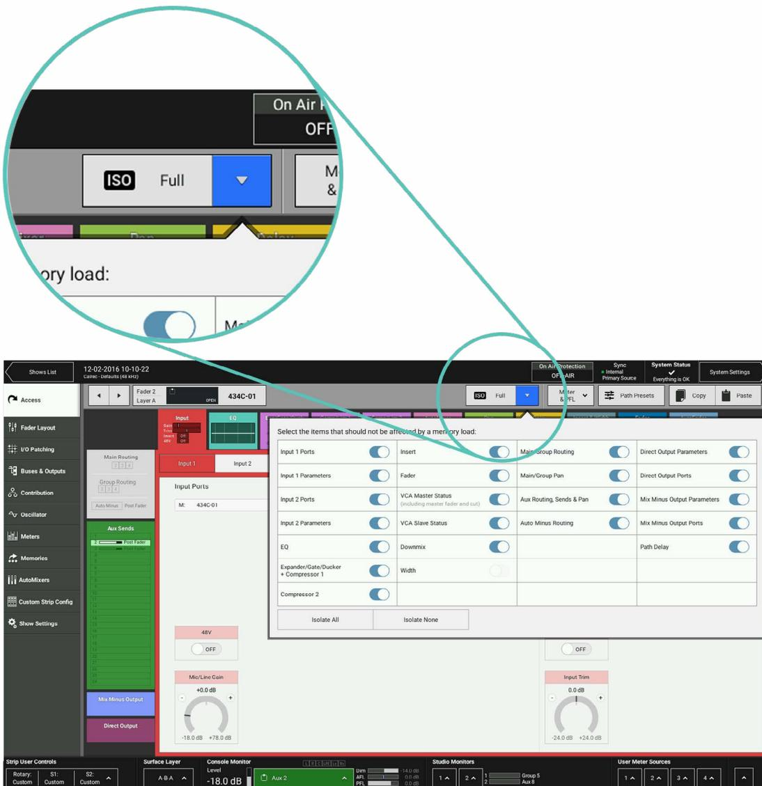
The Isolation status of each path is indicated on its fader display—a blue ISO icon indicates a fully isolated path and a green ISO icon indicates partial isolation is in operation for that path.
