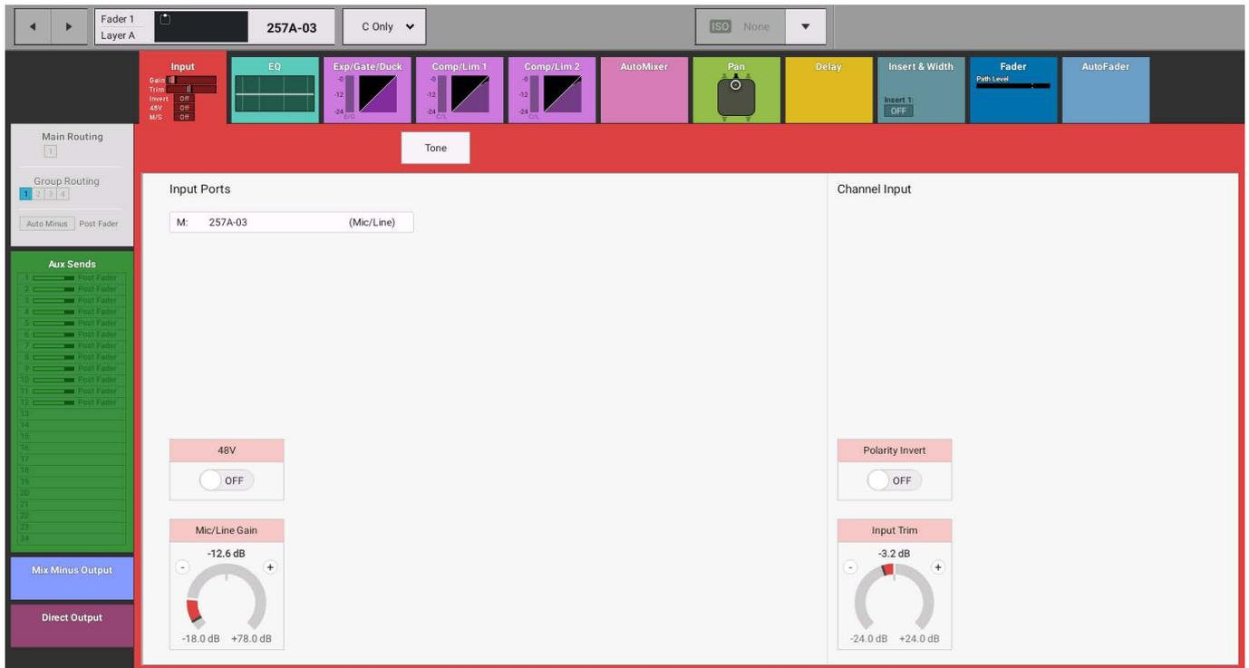
Figure 11 shows the 'Full Path' on the Input page. As this is the 5.1 Channel it shows the combined effect of the changes made on the spill legs. For instance the Mic Gain shows the Highest and Lowest Mic Gain setting made on the spill legs as a combined display.
