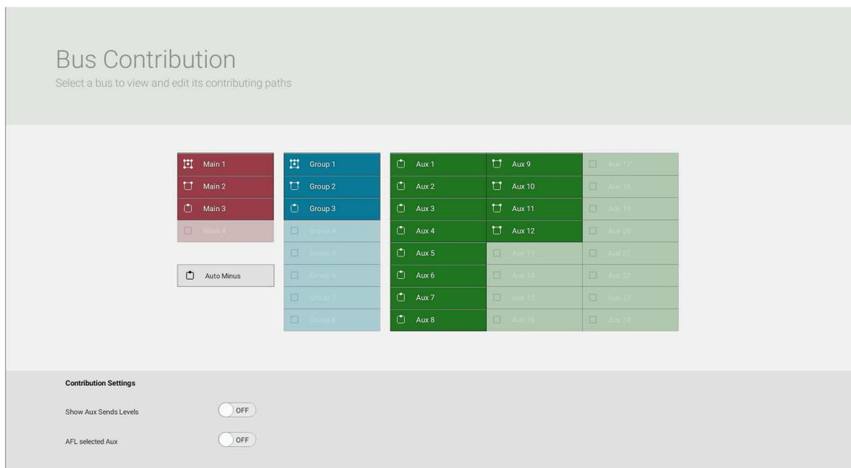
Tap to select any of the bus selectors (mains, groups, auxes or auto minus) in the contribution screen and the fader **ACCESS** buttons for any paths that are currently routed to the selected bus will light as shown in Figure 3. In the following image Group 6 has been accessed in contribution mode. The Global and Strip User buttons can be configured to act as a shortcut to access contribution mode.
