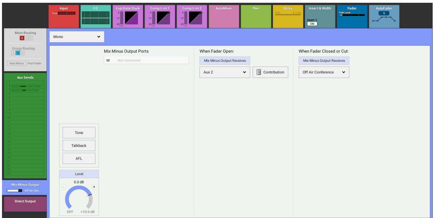
Once the mix minus output has been created there is an option to set different feeds depending on whether the channel/group fader is open or closed.
