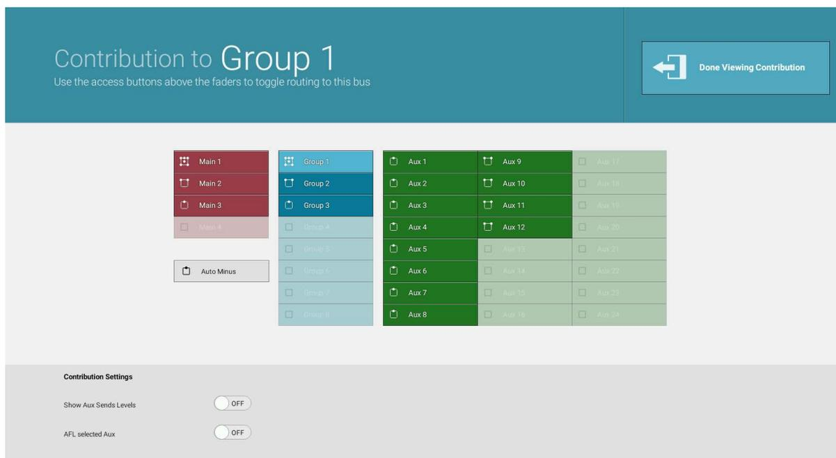
At this point you can toggle on/off the routing of any path to the selected bus by pressing its fader **ACCESS** button.
