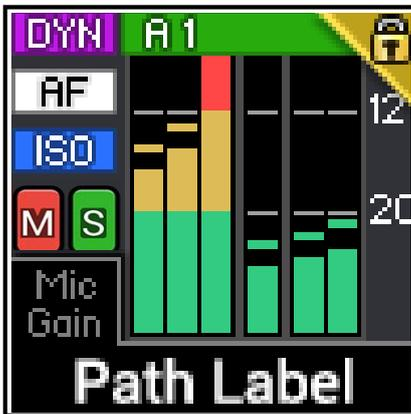
This fader is a secondary master. If a path is attached it is a slave to this secondary master. Push ACCESS to see/alter the level of the slave path.
