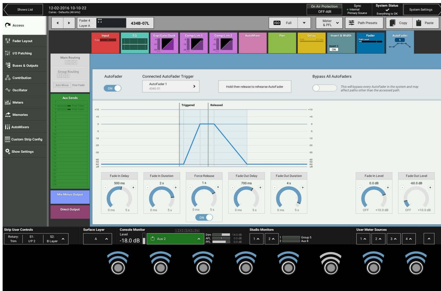
The AutoFader TFT screen gives a visual representation of the behaviour of the AutoFaders position over time and provides information about which AutoFader is in use and which GPI the AutoFader is being triggered from.
