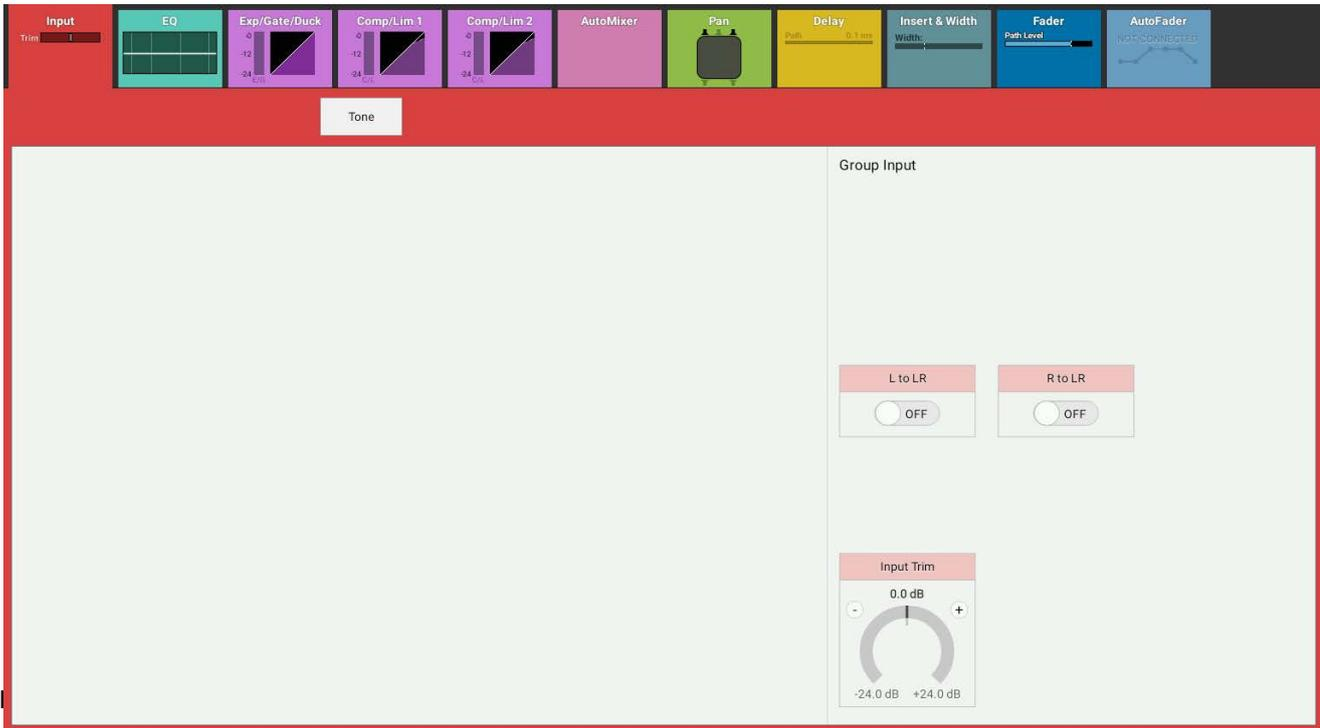
Inputs 1 and 2 have separate input trim controls. These can be linked from the Tools menu on the Access> Input screen as shown in Figure 5. The wording on the Control Cell changes to show the words 'Trims Linked' between the Input 1 and Input 2 source identifiers. The display on the screen also shows the fact that the Input trims are linked.
