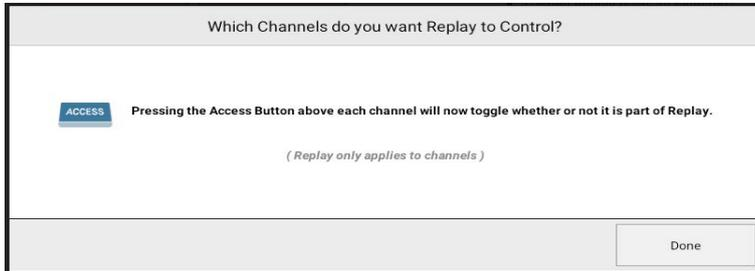
When Replay is active these channels will switch to Input 2, when Replay is turned off the input channels switch back to input 1. Replay makes setting up a virtual sound check easy. With the sources connected to input 1 each source is sent to a recorder and its returns are connected to input 2.
