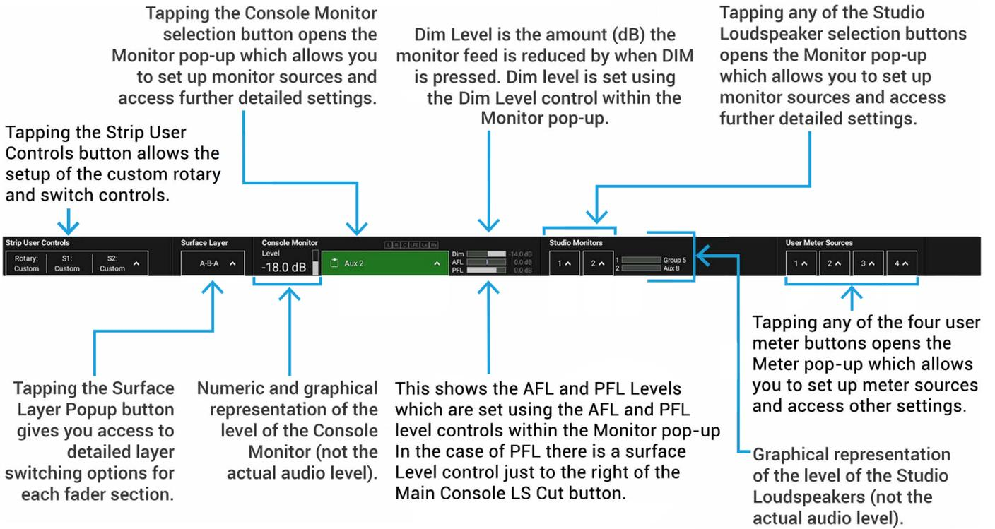
Note: the Console and Studio 1 monitors are surround. If using only a stereo pair of speakers for these monitor, ensure that phantom centre is selected in the options - if this is not done, when mono is pressed on the surface to hear a mono downmix, the user will hear nothing as the mono downmix is routed to centre speaker unless phantom centre is selected.
