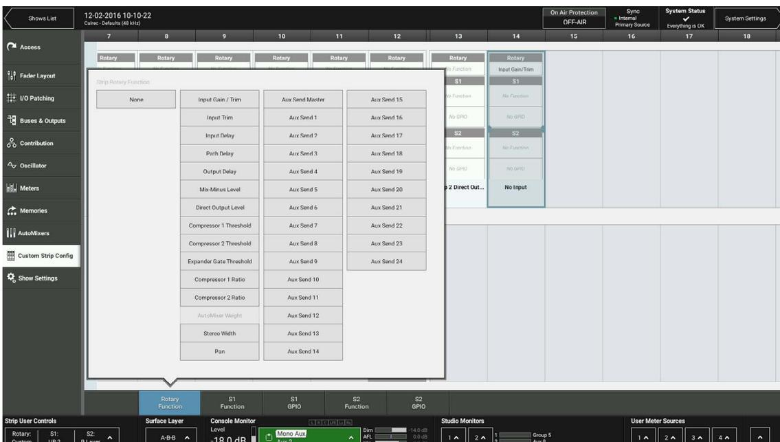
**FIGURE 3 - CUSTOM STRIP CONFIGURATION-S1 AND S2 USER BUTTON FUNCTIONS**
