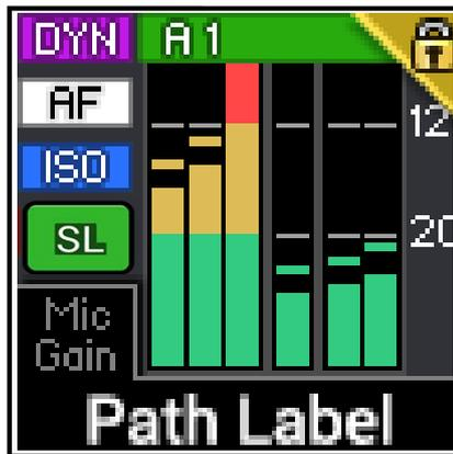
This fader is a slave. If a path is attached, the level of the fader controls the level of the path.
