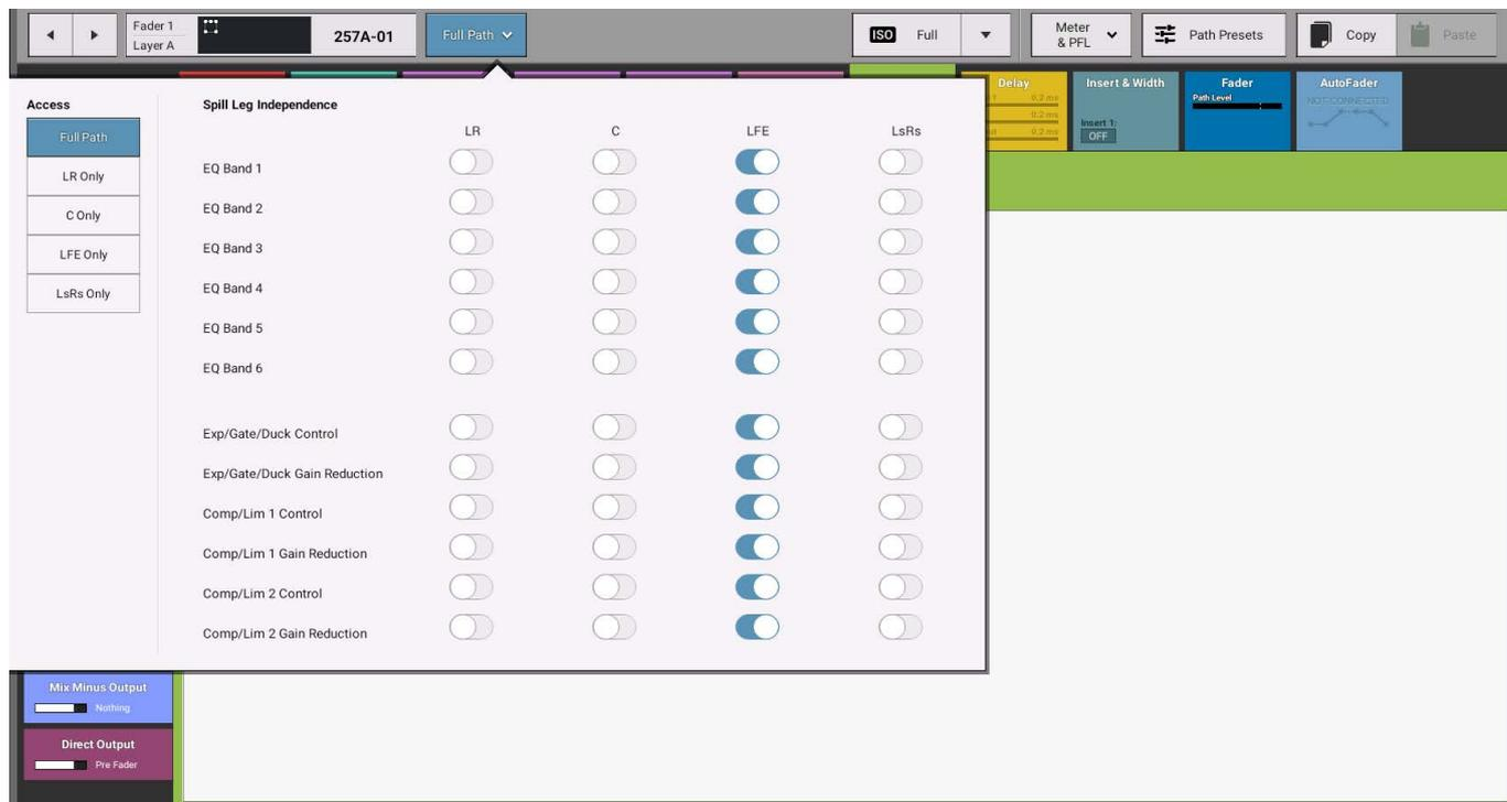
Figure 4 shows the 'LR Only' spill legs on the Pan page. As this is a Stereo spill leg all the controls that would normally appear for a Stereo path are made available. The 'LsRs' spill leg appears with the same stereo parameters controls as shown here for the LR spill legs.
