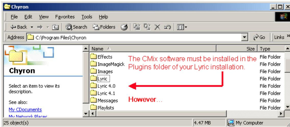
The system pictured here contains different versions of Lyric. In the first illustration below, the installation script did not place the file in the appropriate directory. The operator's intent here is to use CMix with Lyric Version 4.1.
