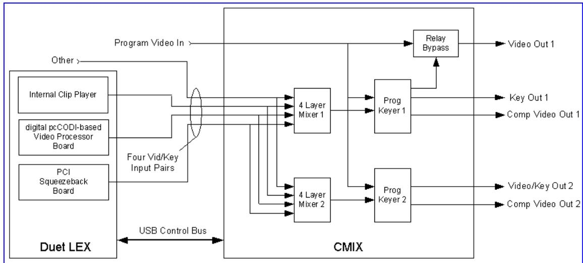
**Example of CMix connected to Duet LEX for USB control and 3 video sources**
