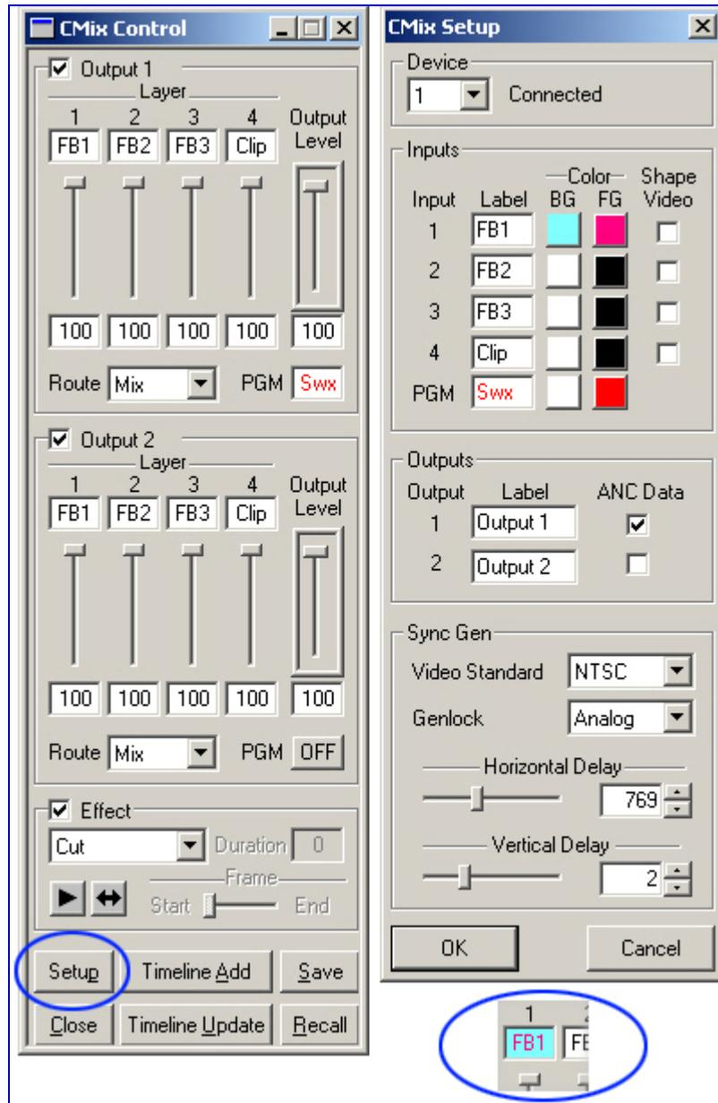
**CMix's main controls (left) and controls-setup panel (right)**
