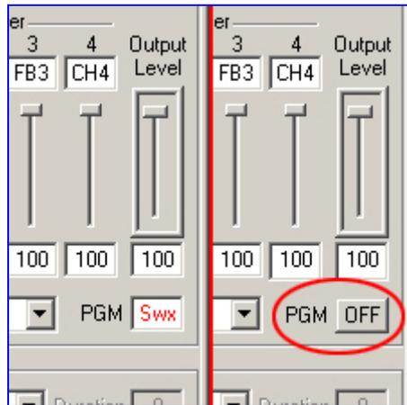
**The Program input can only be assigned to a source or turned off.**
