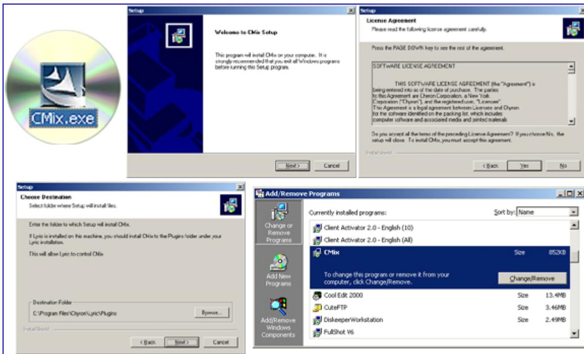
CMix's plugin software for Lyric is installed by the familiar Install Shield process. Locate the **CMix.exe** on the included CD and double-click it. The install process begins. Follow the instructions in the installation script, and click **Next** as needed. (To uninstall the CMix software, use the Windows Add/Remove Program facility, as seen in the lower right corner of the illustration above.)
