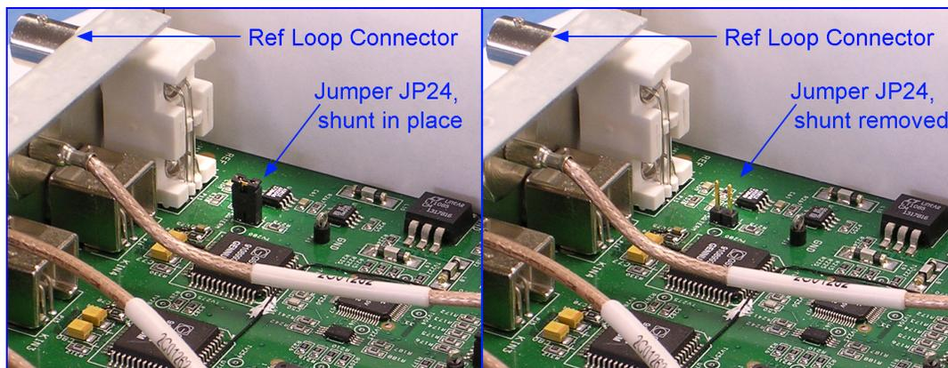
**Remove the shunt at jumper JP24 to share analog genlock**
