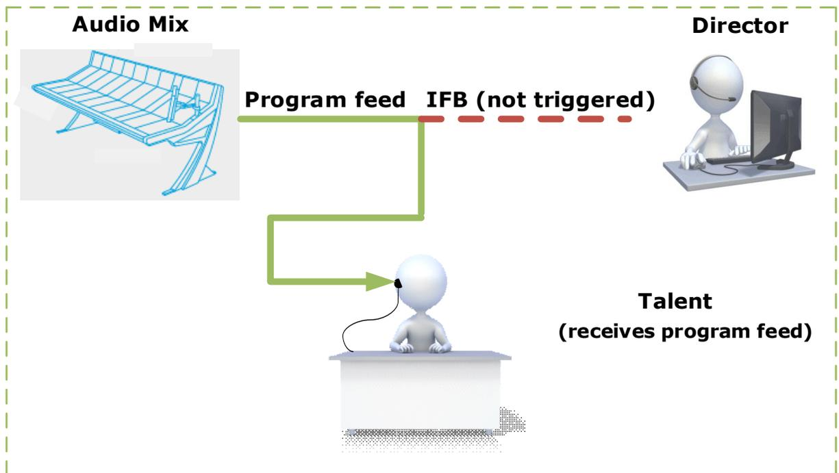
Figure 4-25 Broadcast scenario with no IFB trigger.
