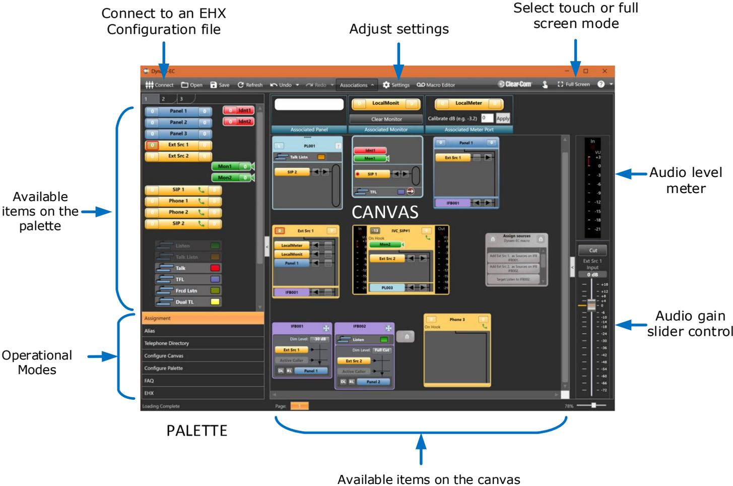
Figure 4-1: Quick reference to the Dynam-EC screen
