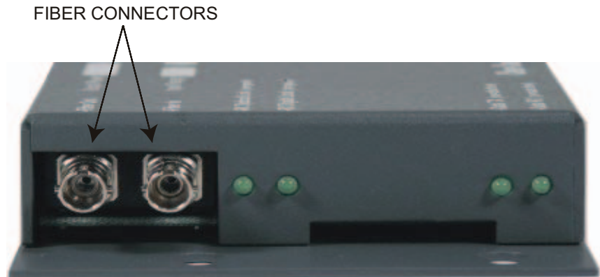
Figure 2-1: ST Optical Connections on an FIM-202D Unit's Front Panel
