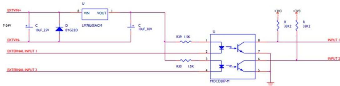
**Figure 9: Opto-Isolated connection to Eclipse HX-PiCo GPI connector**
