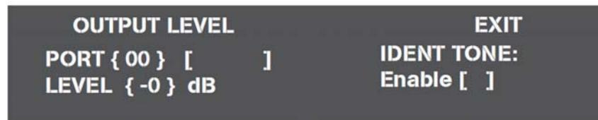
Figure 21: Output Level menu display
