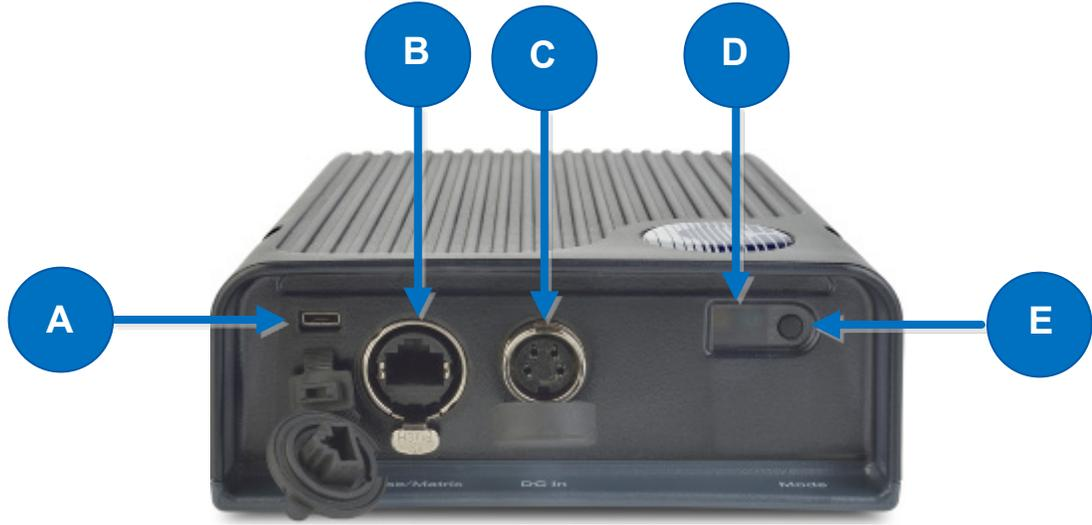
Figure 6-2 FS II Transceiver/Antenna Connector Panel
